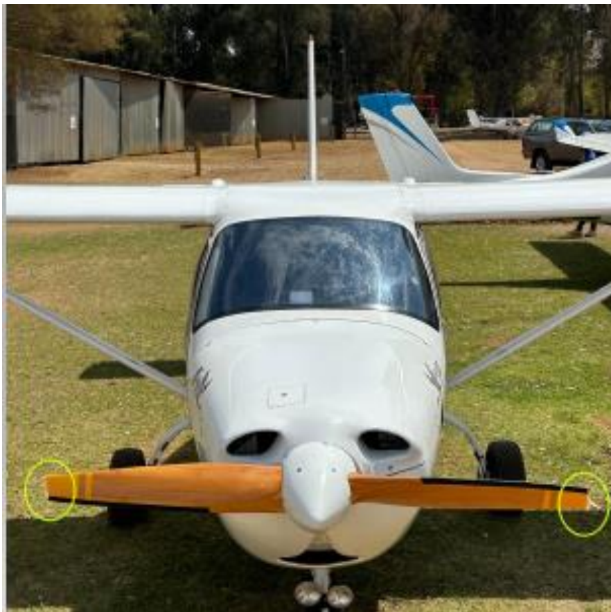
Figure 2: Yellow circles indicate the damaged propeller tips. (Source: Owner)
