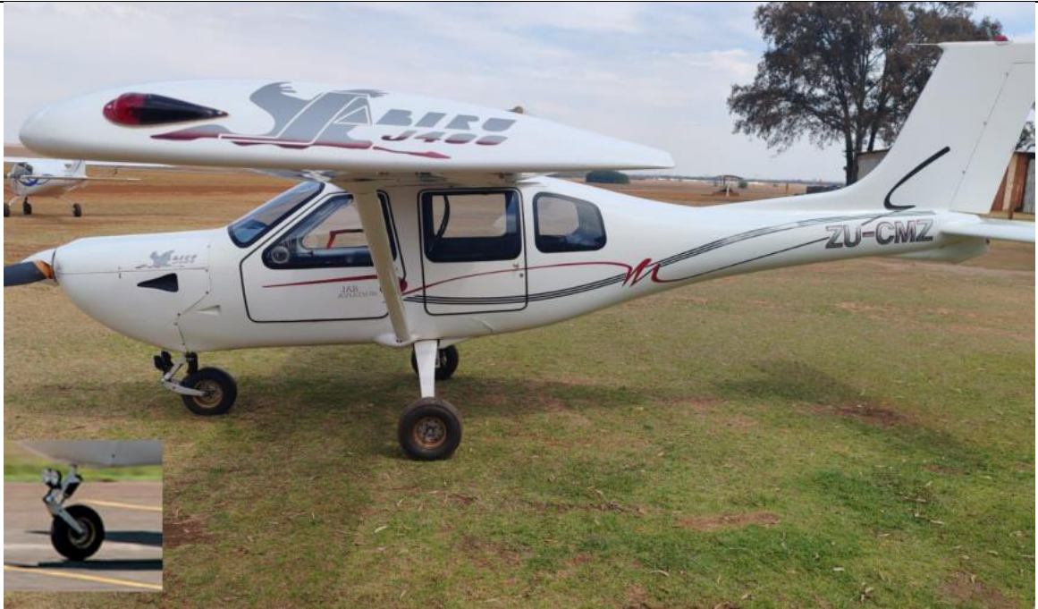
Figure 1: The damaged nose gear. The inset shows an undamaged nose gear. (Source: Owner)
