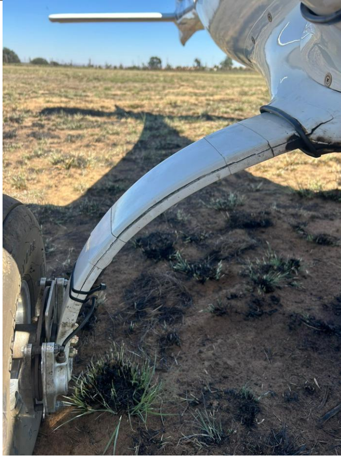
Figure 3: The delaminated strut. (Source: Pilot)
