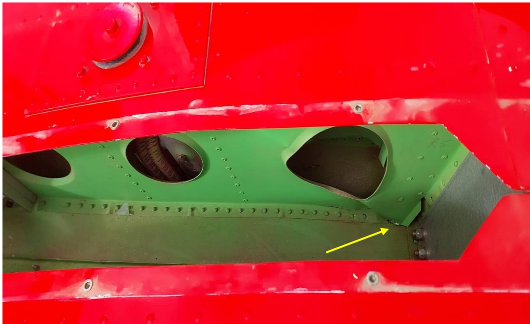
Figure 5: Damage sustained to the left side of the main gear landing gear box. (Source: Pilot)
