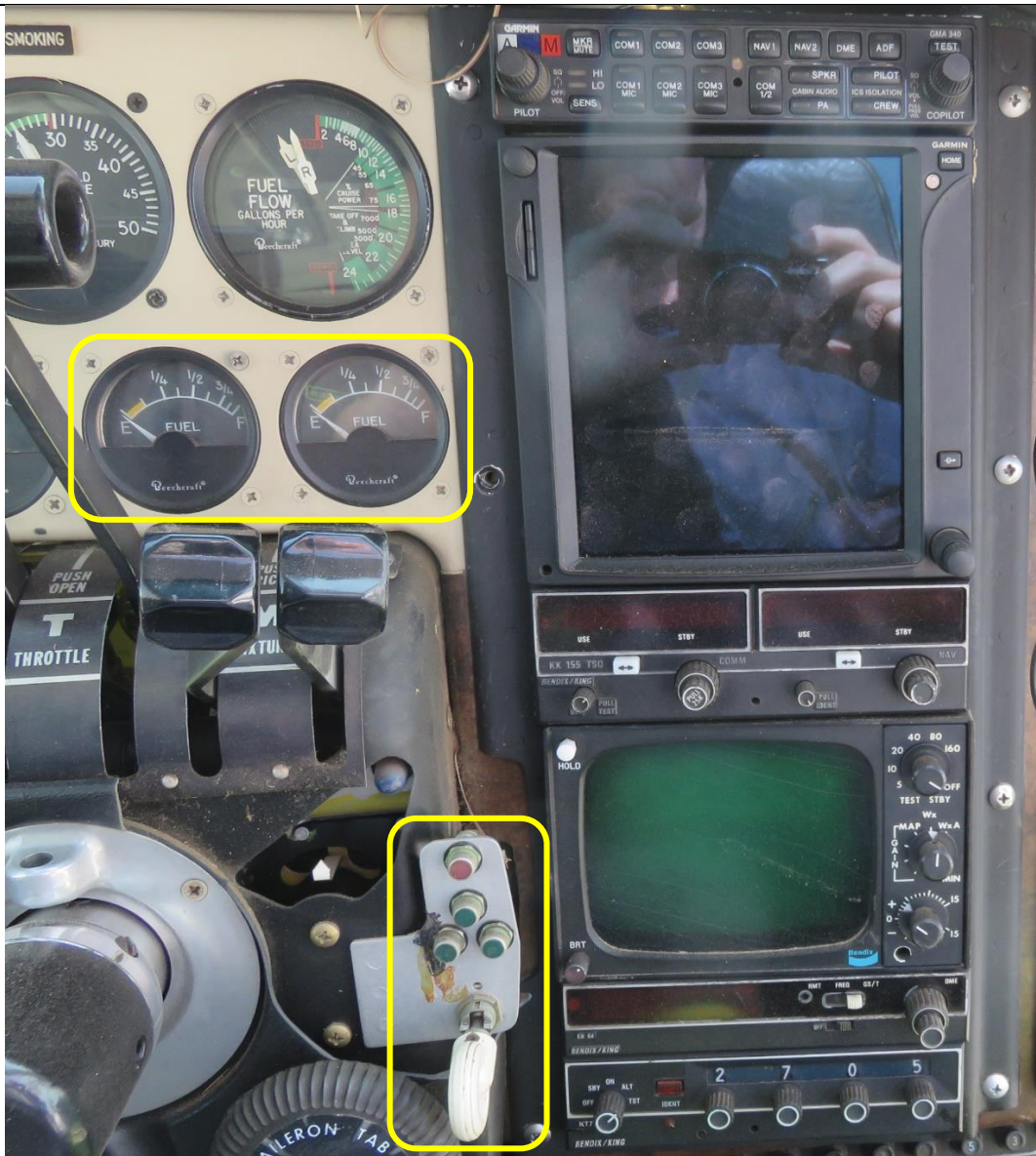
Figure 7: The fuel gauges in the cockpit with the landing gear lever in the DOWN position.
