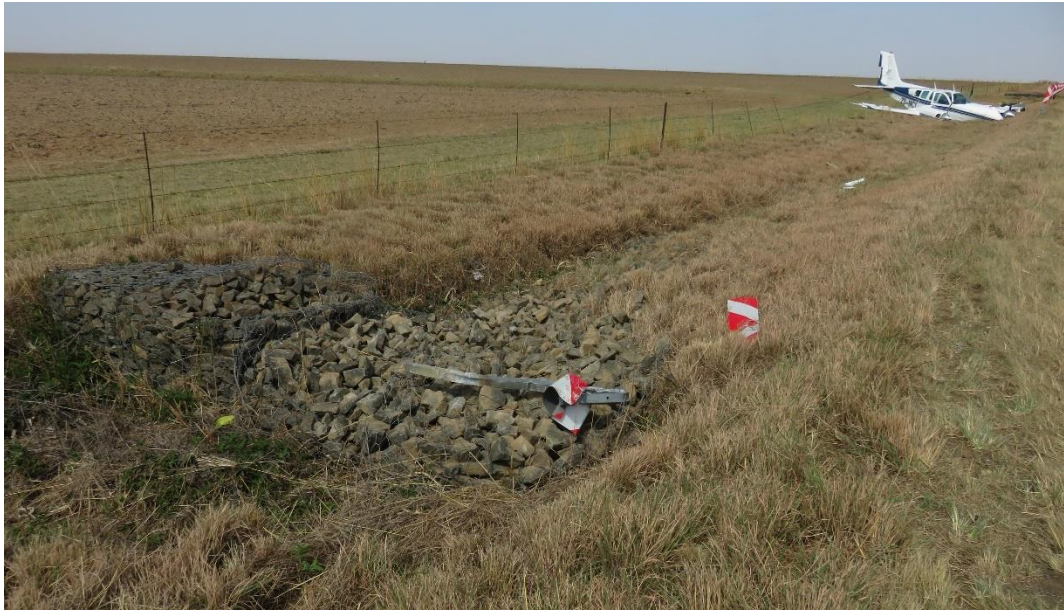
Figure 2: The stormwater barrier and two of the hazard marker boards that the aircraft impacted.
