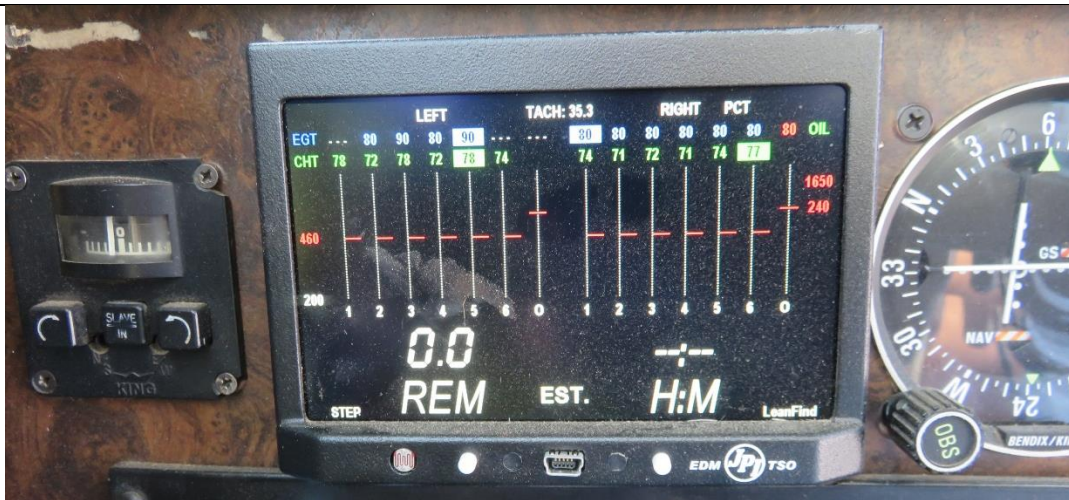
Figure 9: The JPI EDM 790 unit that was installed in the aircraft.
