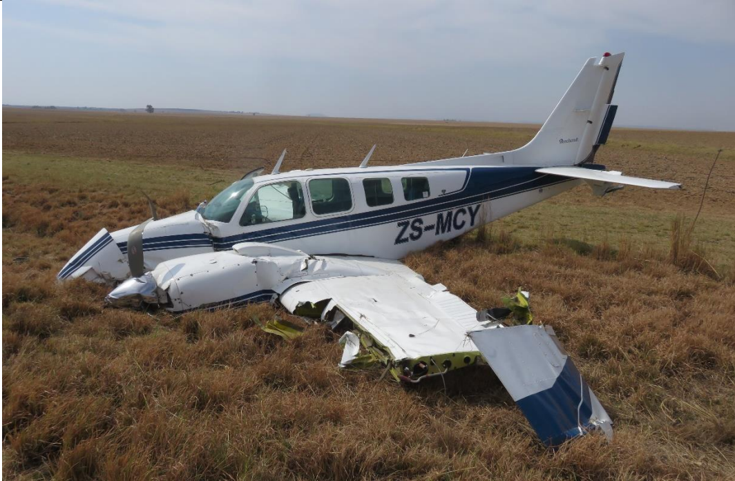
Figure 4: Substantial damage to the left wing.
