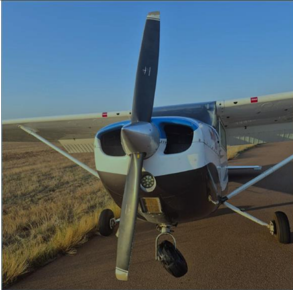
Figure 2: Damage sustained to the nose gear and the propeller blades. (Source: FAWB-ARFF)
