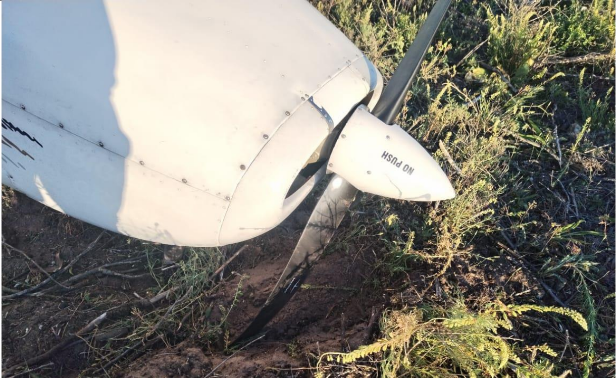
Figure 3: The bent propeller blade. (Source: Operator)
