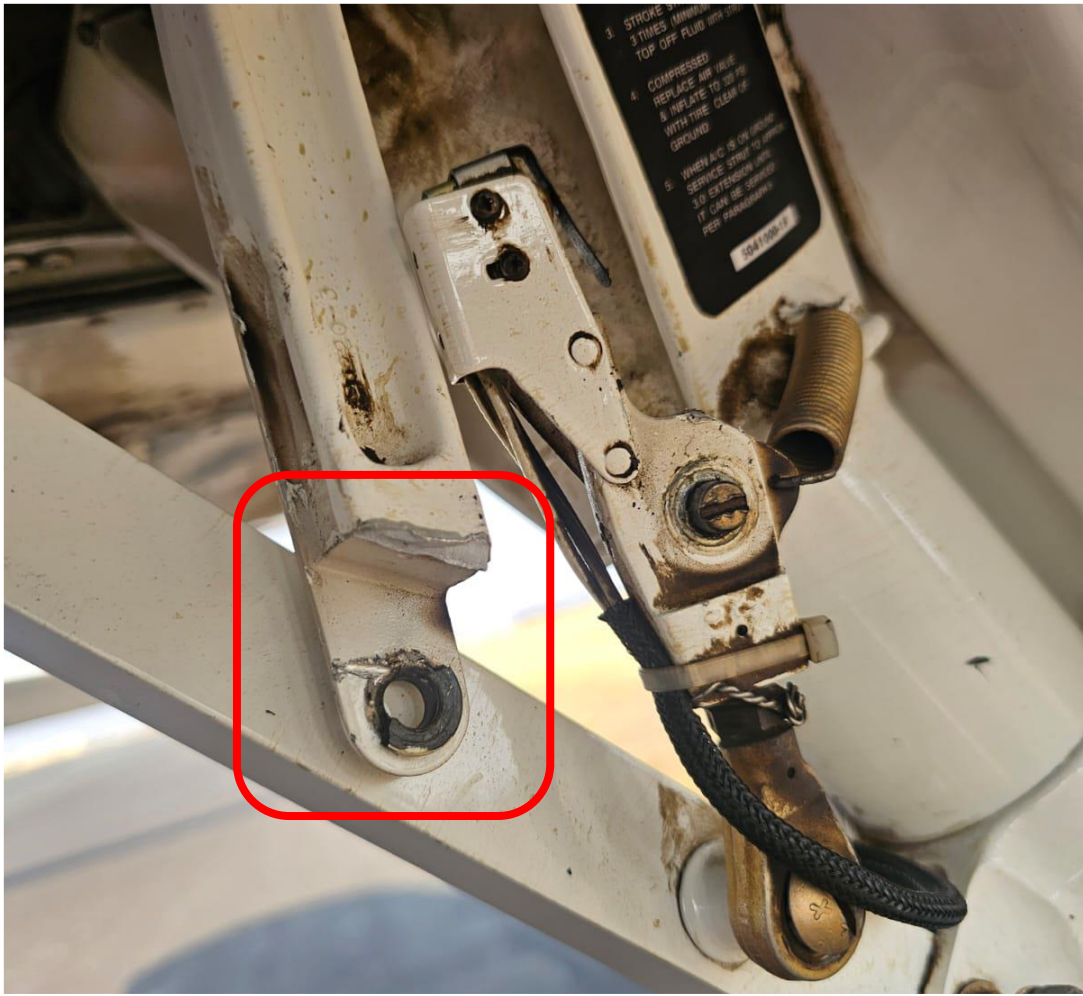
Figure 6: The broken lug on the bell crank assembly. (Source: AMO)
