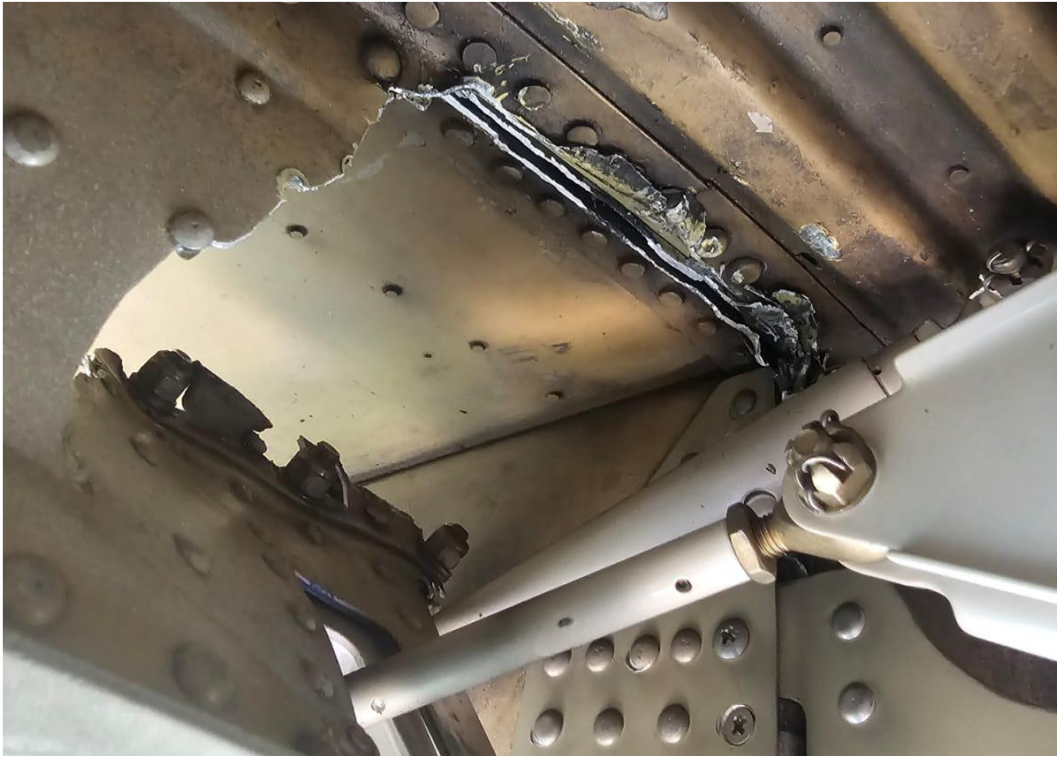
Figure 8: Some structural damage to the left wing. (Source: AMO)
