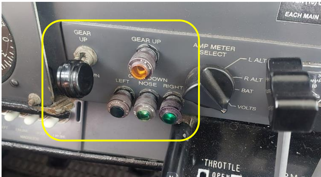
Figure 10: The landing gear lever and indication lights in the cockpit.
