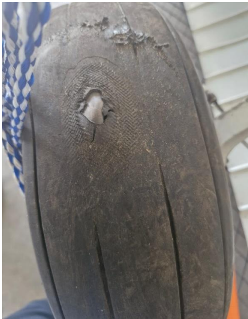
Figures 3 and 4: Damage on the aircraft's left and right main wheel tyres due to excessive braking.
