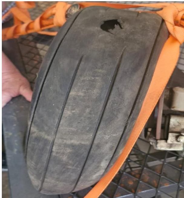
Figures 3 and 4: Damage on the aircraft's left and right main wheel tyres due to excessive braking.
