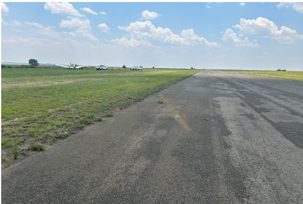
Figure 2: Tyre markings on the runway indicate the point at which the aircraft veered off to the left. (Source Pilot)
