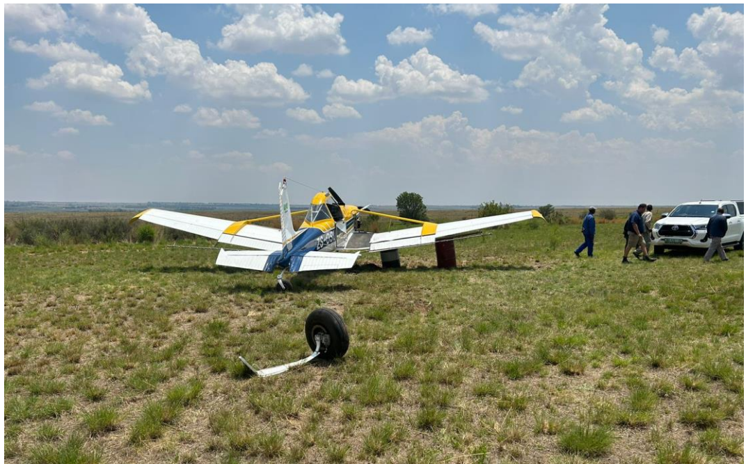
Figure 4: The right main landing gear strut and wheel assembly that broke off. (Source: Pilot)
