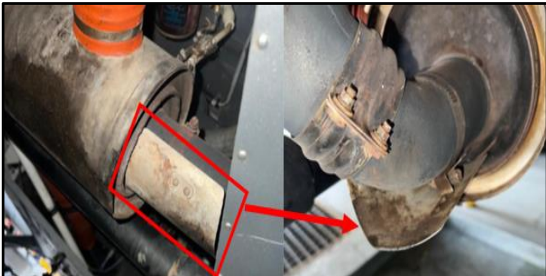
Figure 5: The muffler shield on the right side of the helicopter (left) and a muffle taken from a different angle (right).
