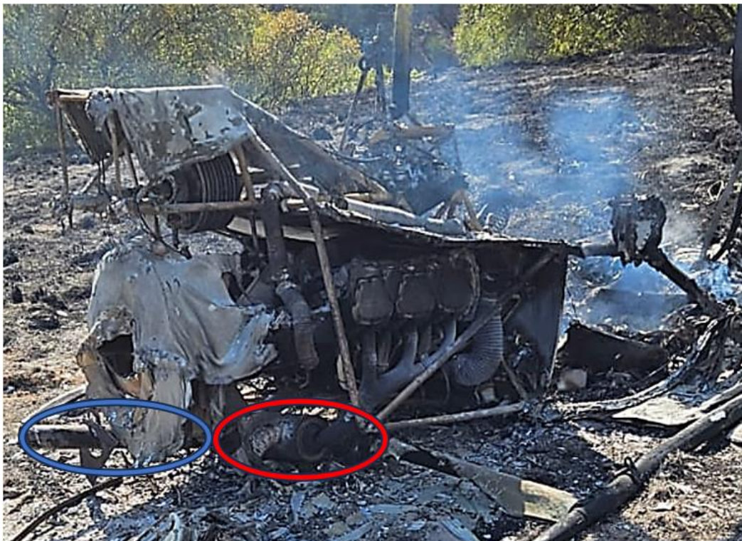
Figure 2: The wreckage. The blue circle shows the exhaust tailpipe (blue circle), and the red circle depicts the exhaust pipeline (red circle) with no shield and muffler.
