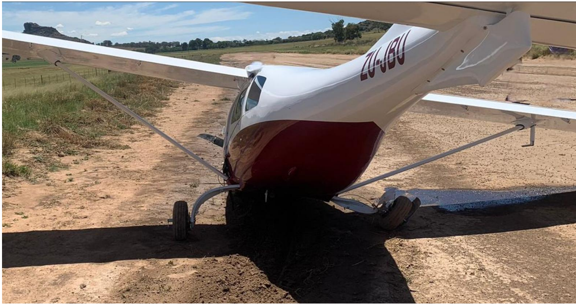
Figure 3: The rear view of the aircraft showing the damaged right main gear. (Source: Pilot)
