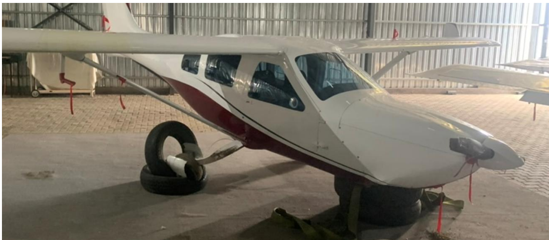
Figure 4: Right view of the aircraft showing the damaged right main gear strut. (Source: Pilot)
