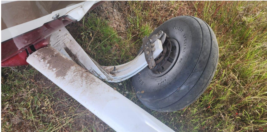
Figure 4: The collapsed right main landing gear. (Pilot)
