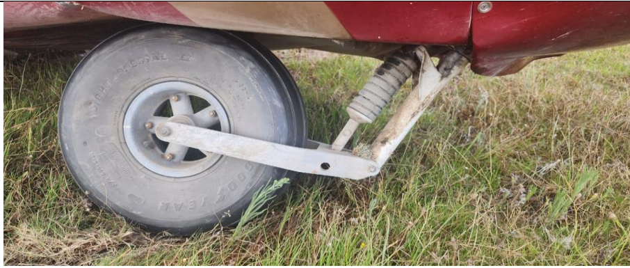
Figure 3: The collapsed nose gear strut. (Pilot)
