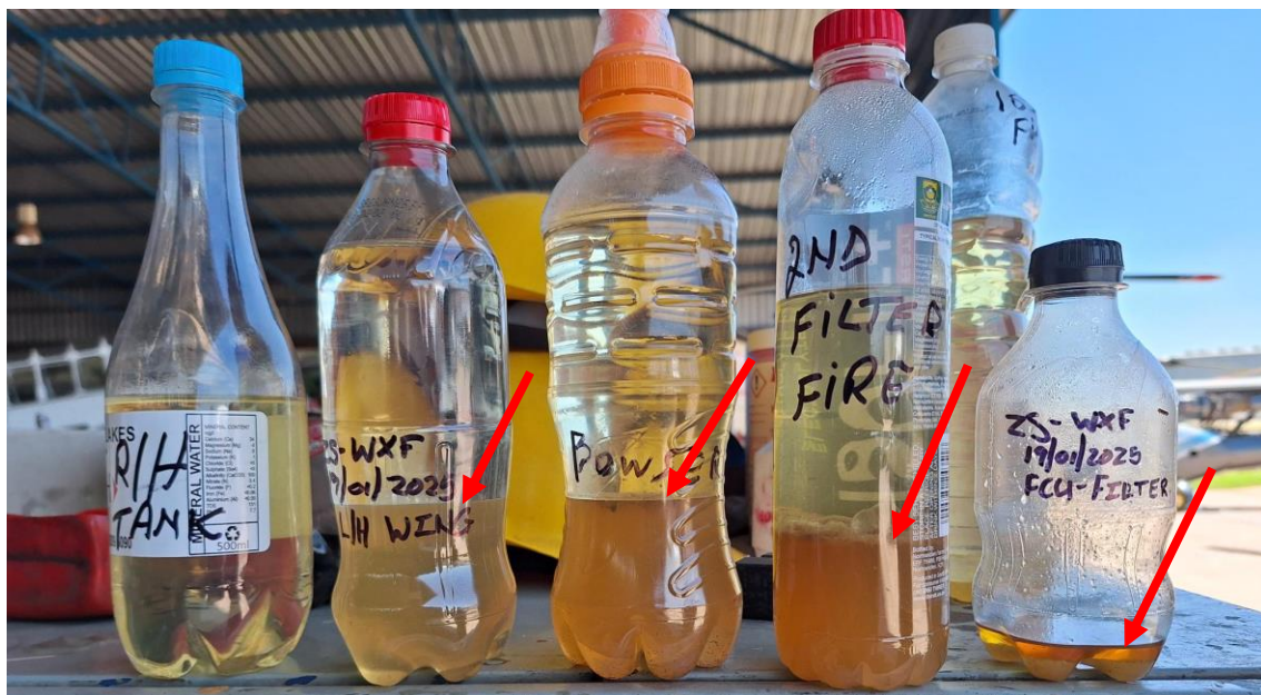
Figure 7: The fuel samples taken a day after the accident. The red arrows indicate the contamination in the fuel.
