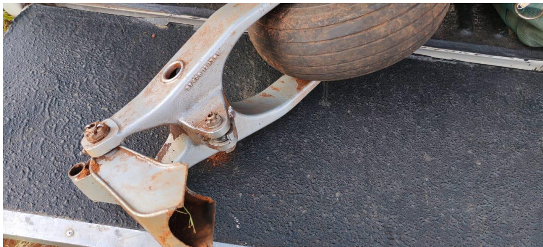
Figure 4: The tail wheel assembly that broke off at the welded lug. (Source: Pilot)
