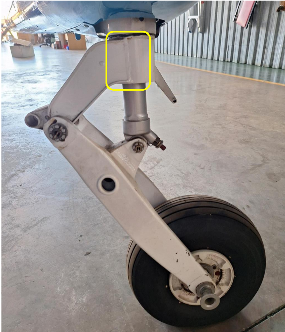
Figure 5: Tail wheel assembly of a similar aircraft. The failure occurred on the welding surface area that is highlighted in yellow.
