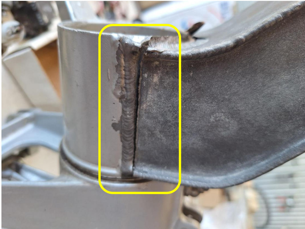
Figure 6: The welded area that failed on the tail wheel assembly. This is the actual tail wheel assembly that was fitted to the aircraft and failed during the forced landing.
