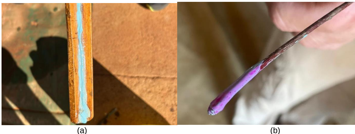
Figure 15: The paste on a dipstick (a). The paste changes colour when water is detected (b).
