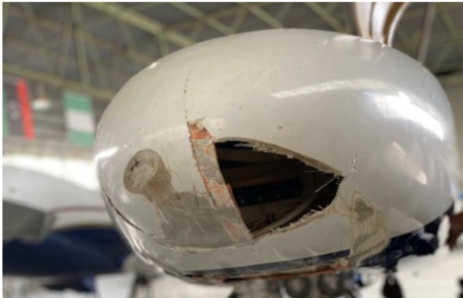
Figure 3: The damaged nose cone. (Source: Pilot)
