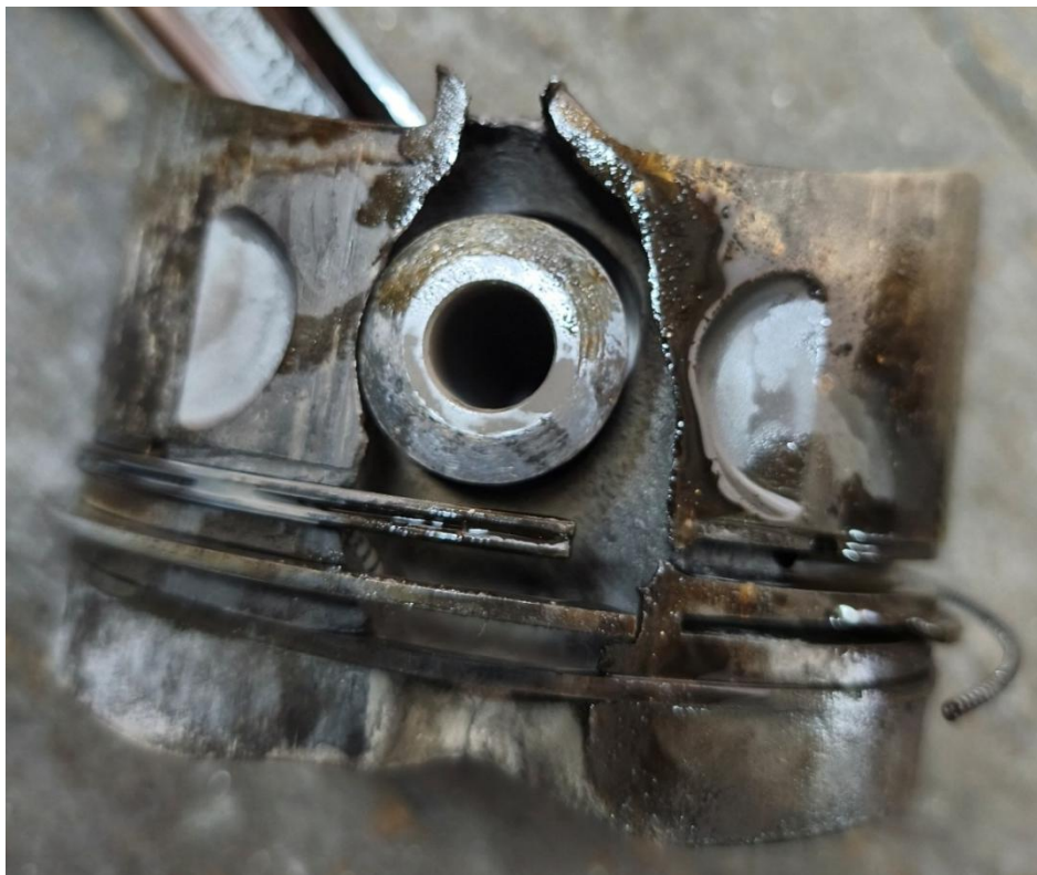
Figure 2: The failed engine piston pin plug from the damaged Number 3 piston.
