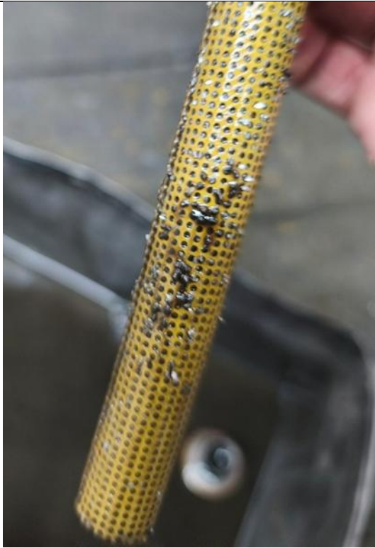
Figures 3 and 4: Metal particles on the oil pump suction screen and tubing. (Source: Investigator)
