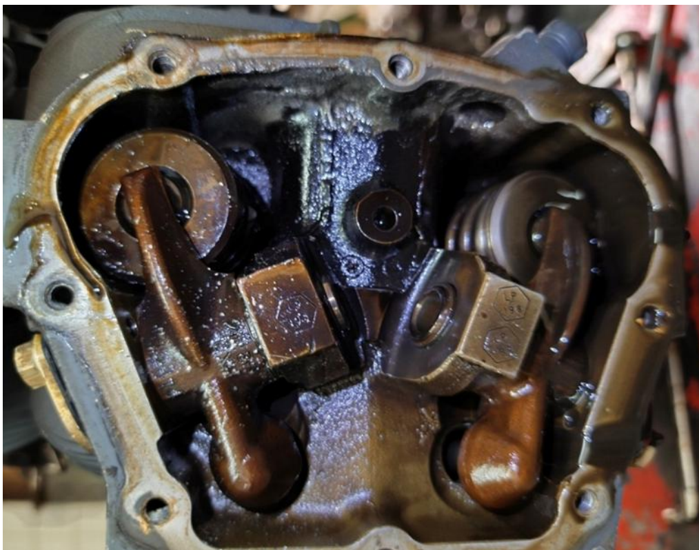
Figure 5: Metal particles found on engine cylinder valves and rocker assemblies due to the circulated contaminated oil.
