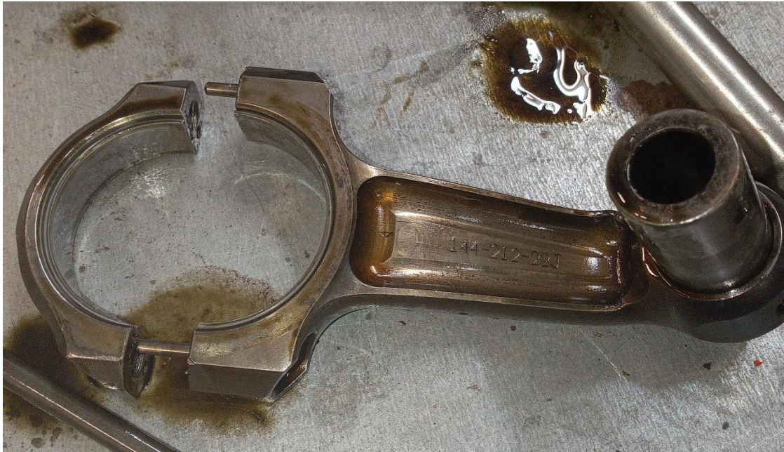
Figure 9: The damaged cylinder Number 6 connecting rod.
