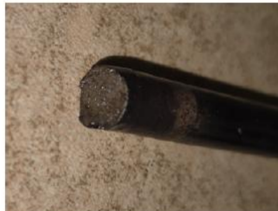
Photo 6: Fracture surface B, exhaust valve
