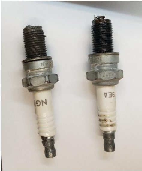
Figures 6 and 7: The damaged spark plugs (left) and cylinder head with the missing exhaust valve.
