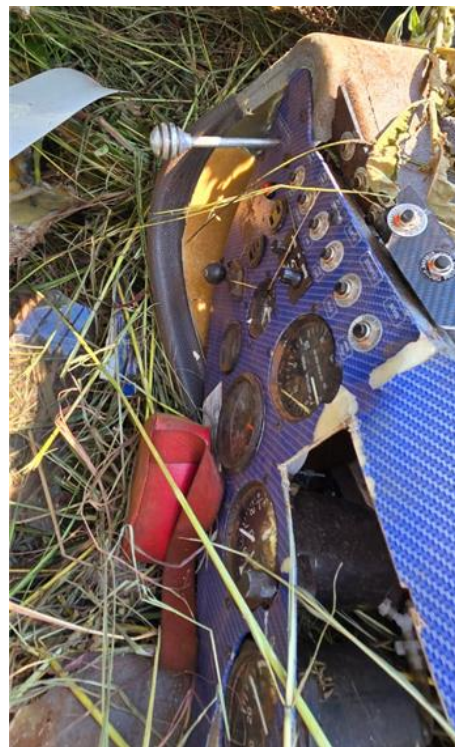
Figures 3 and 4: The damaged left-wing tip and instrument panel (left). The pulled back power lever (right).
