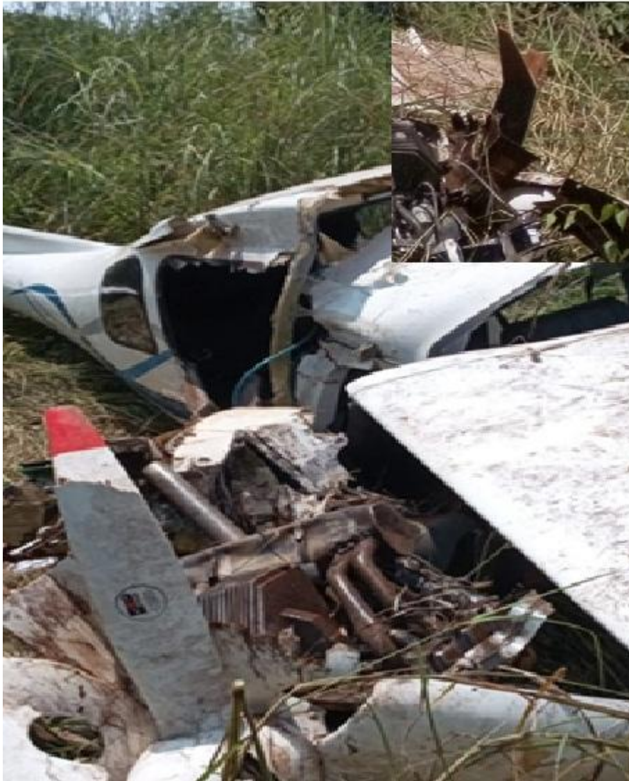
Figure 5: The main fuselage after the accident. Inset picture shows the broken propeller.
