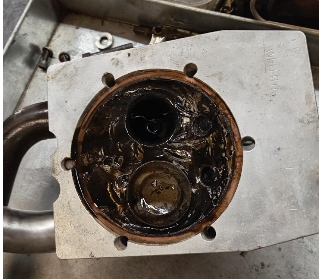
Figures 6 and 7: The damaged spark plugs (left) and cylinder head with the missing exhaust valve.
