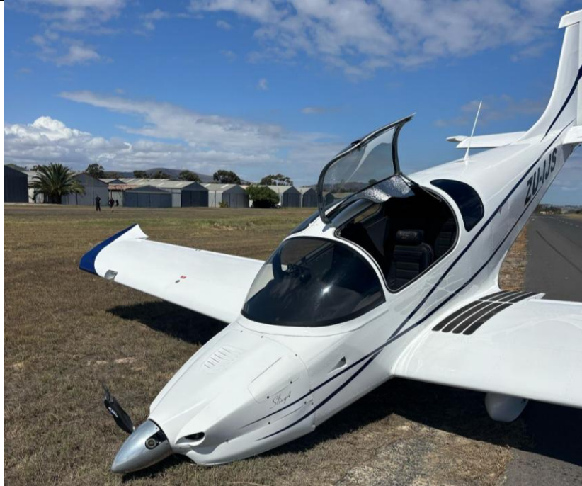
Figure 2: The aircraft on the right-side shoulder of Runway 02 with a damaged nose landing gear and propeller. (Source: Pilot)
