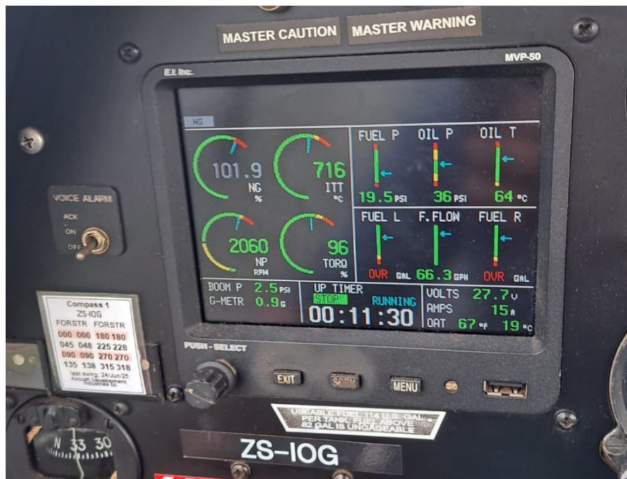
Figure 5: The MVP-50T screen indicates the engine parameters on take-off: interstage turbine temperature (ITT) at 716, prop RPM at 2 060, torque at 96psi, fuel pressure at 19.5psi, oil pressure at 36psi, fuel flow at 66.3gph and oil temperature at 64° Celsius; all parameters were within limits. (Source: Operator)
