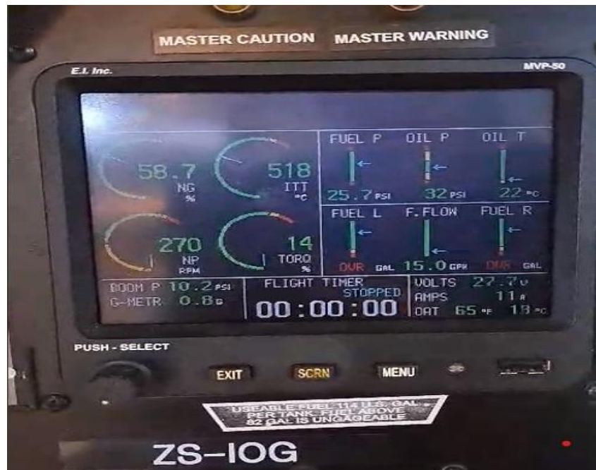
Figure 4: The MVP-50T screen indicates the engine parameters at idle: Normal start and the engine idled at 58.7%, prop revolutions per minute (RPM) at 270, torque at 14 pound per square inch (psi), fuel pressure at 25.7psi, oil pressure at 32psi, fuel flow at 15 gallons per hour (gph) and oil temperature at 22° (degrees) Celsius; all parameters were within limits. (Source: Operator)
