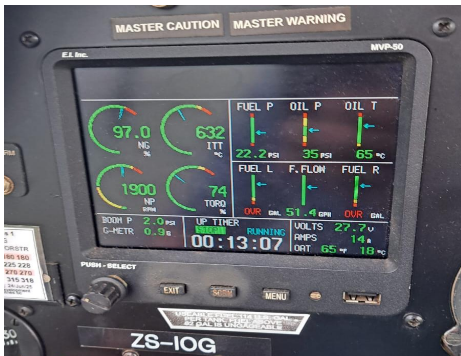
Figure 6: The MVP-50T screen indicates the engine parameters at cruise: ITT at 632, prop RPM at 1 900, torque at 74psi, fuel pressure at 22.2psi, oil pressure at 35psi, fuel flow at 51.4gph and oil temperature at 65° Celsius; all parameters were within limits. (Source: Operator)
