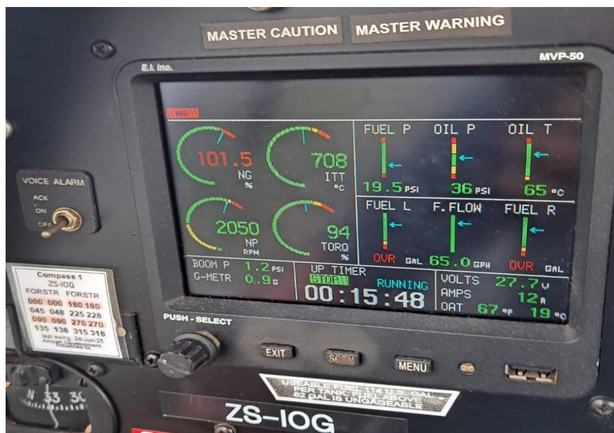
Figure 7: The MVP-50T screen indicates the engine parameters during emergency: ITT at 708, prop RPM at 2 050, torque at 94psi, fuel pressure at 19.5psi, oil pressure at 36psi, fuel flow at 65 gph and oil temperature at 65° Celsius; all parameters were within limits. (Source: Operator)
