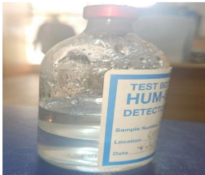
Figure 3: The Hum-Bug test came up negative for water or bacterial growth. (Source: Operator)
