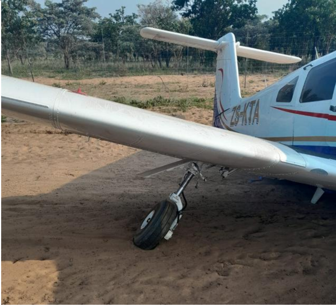
Figure 4: The bent oleo after the accident. (Source: Pilot)
