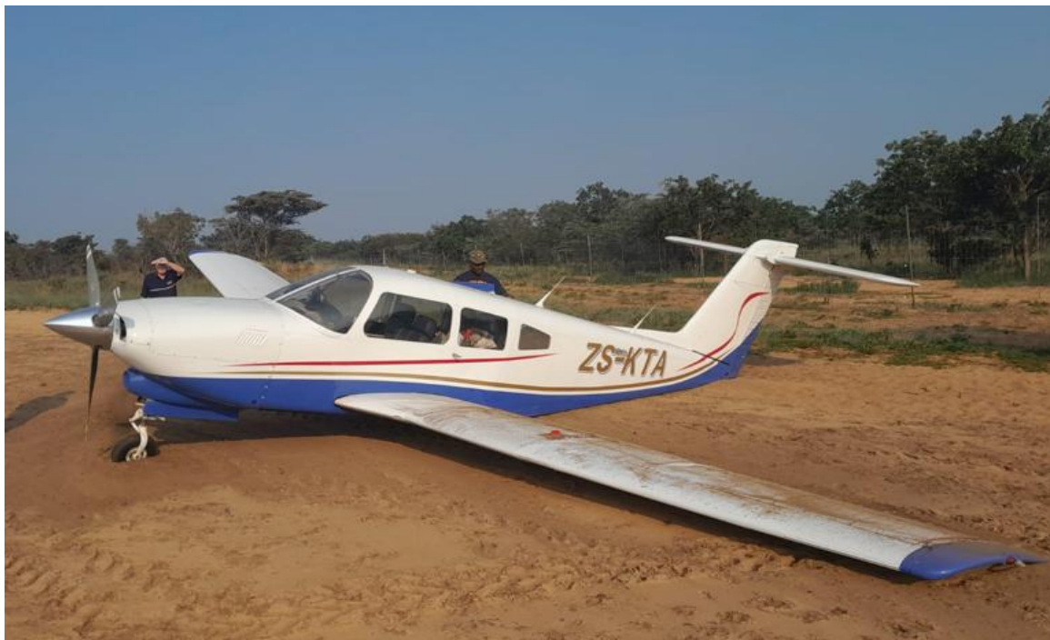
Figure 3: The left wing and the aft fuselage resting on the runway post-accident. (Source: Pilot)
