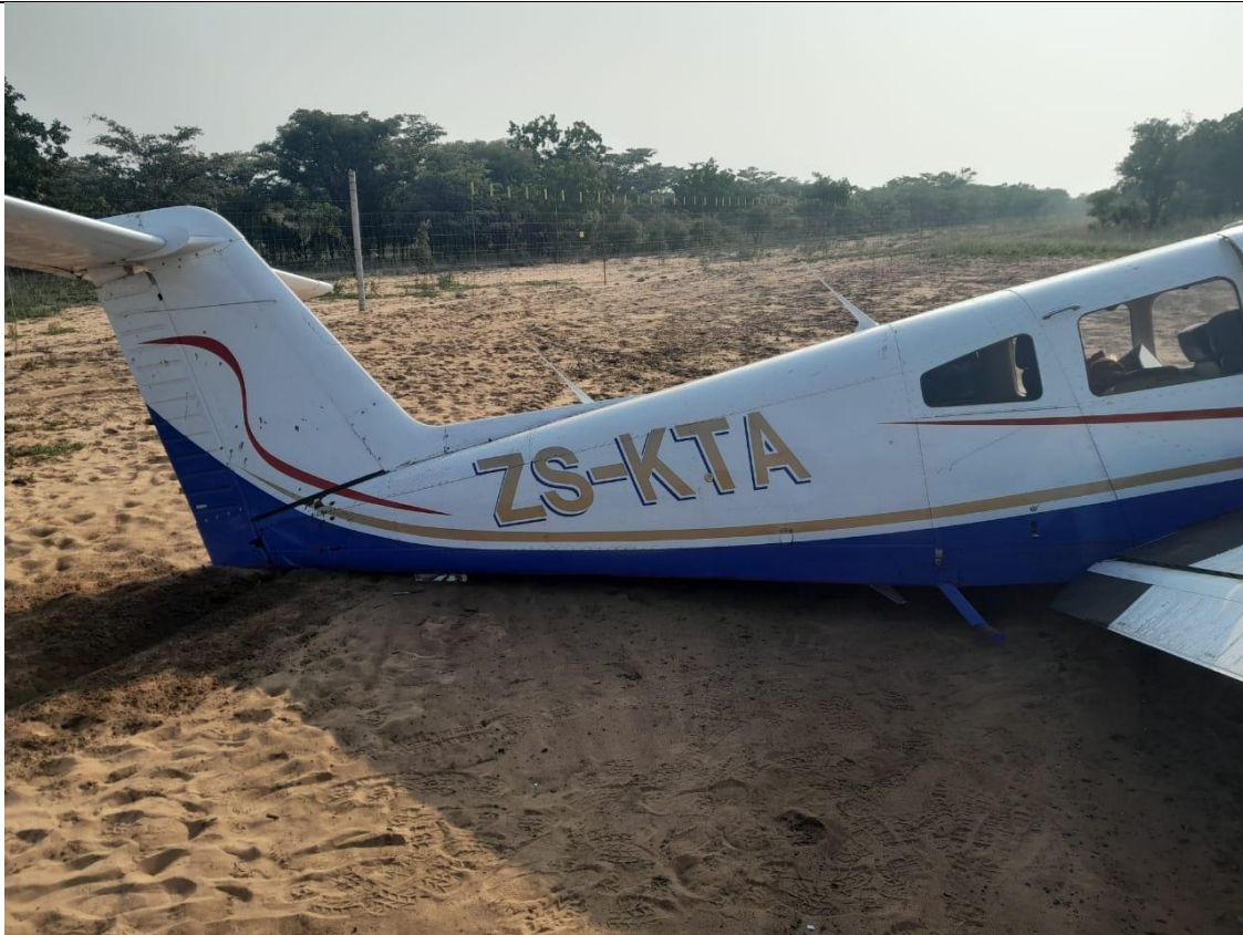
Figure 2: The collapsed landing gear on the soft sand-covered runway. (Source: Pilot)
