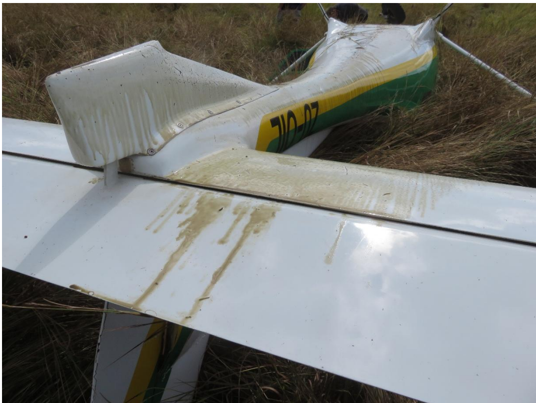
Figure 5: The lower fuselage and left horizontal stabiliser and elevator covered with engine oil.
