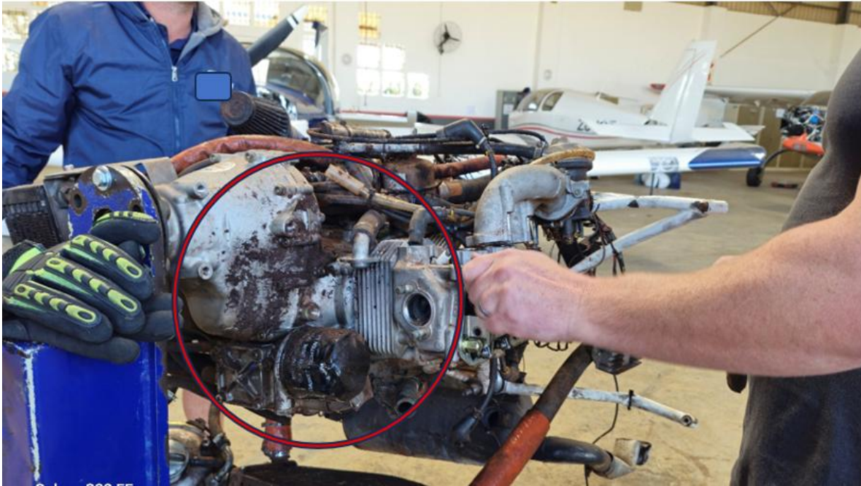
Figure 9: Damage on the left side of the engine.
