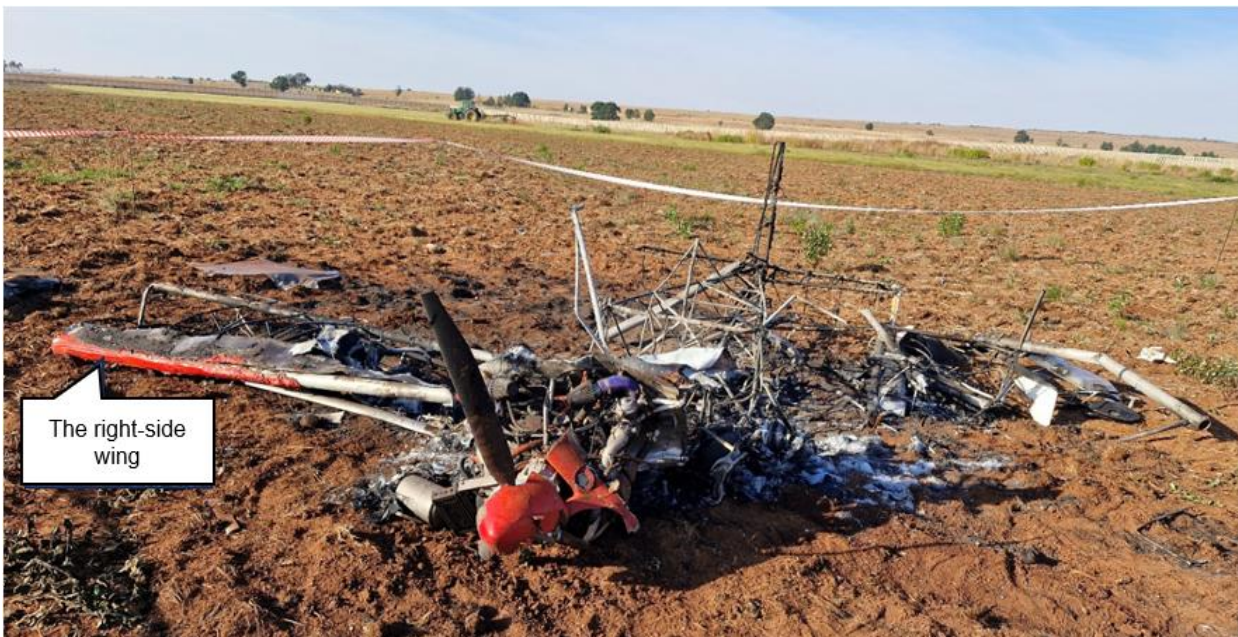
Figure 6: The condition of the right-side wing.
