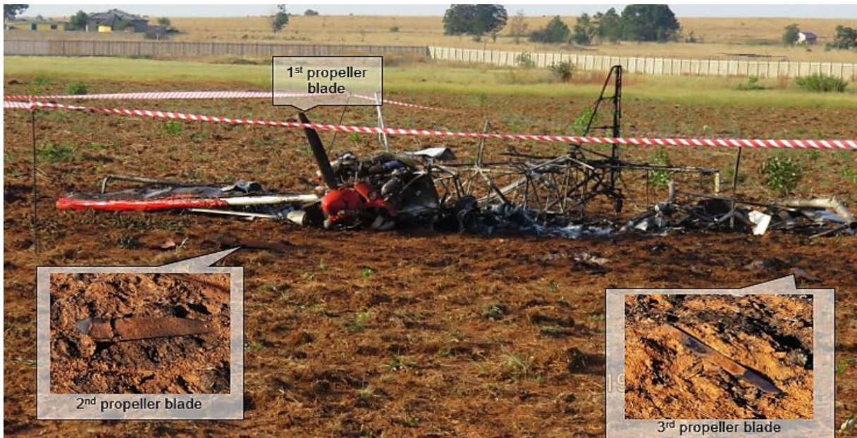
Figure 7: The positions of the broken propeller blades after the accident.
