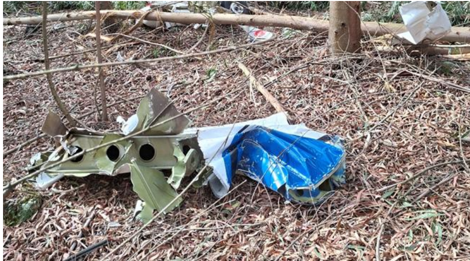
Figure 5: Exposed spar and a portion of the severed wing.
