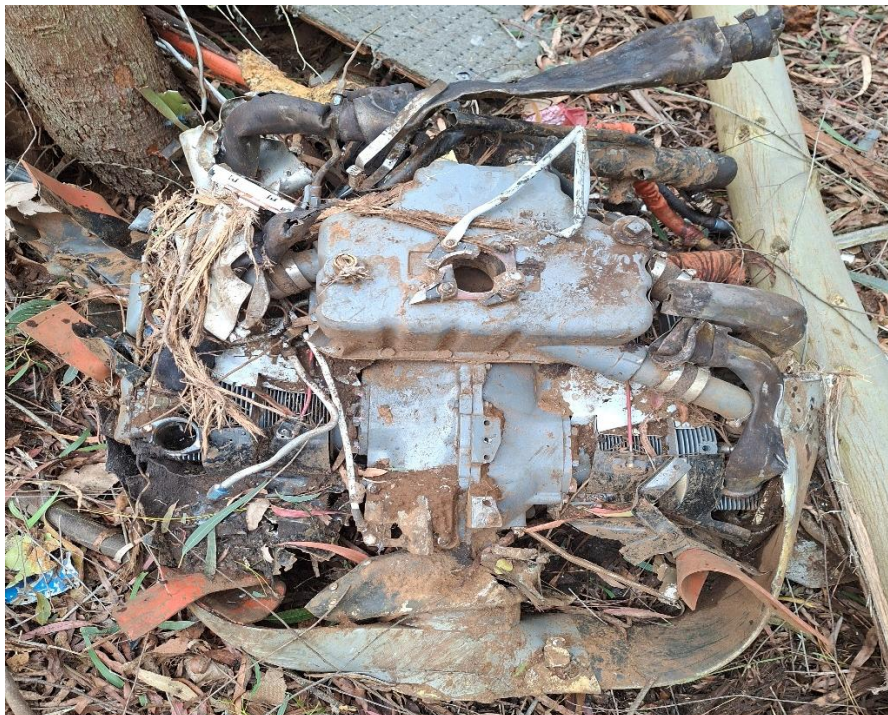
Figure 8: The inverted engine with the propeller blade tip that was severed.
