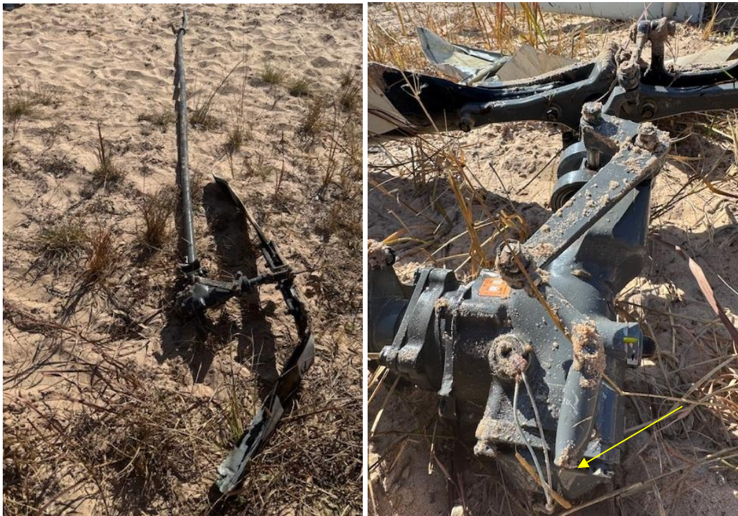
Figures 9 and 10: The separated tail rotor drive shaft and blades (left picture); and the broken pitch change bellcrank (right picture).
