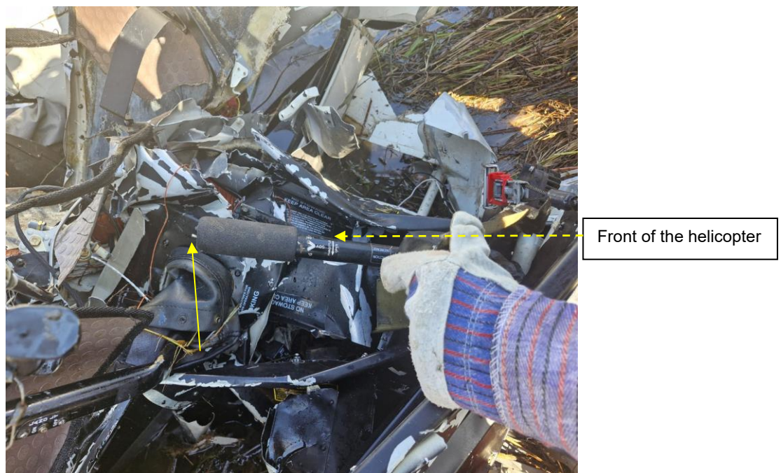
Figure 12: The collective pitch control lever near the full UP position and the engine governor in the ON (UP) position (yellow arrow).
