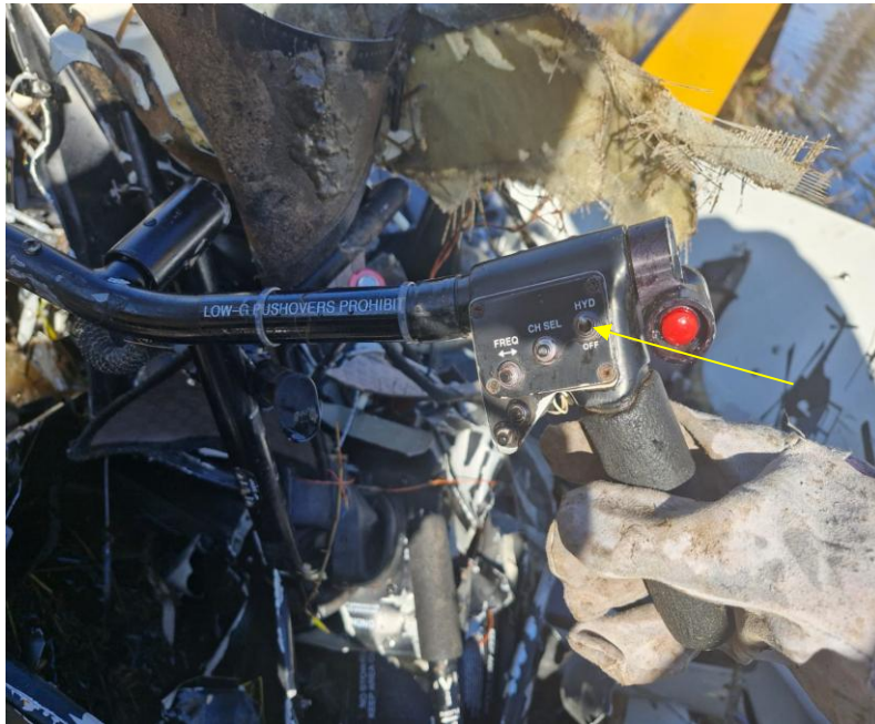
Figure 11: The cyclic pitch control lever indicating the hydraulic switch in the ON position.
