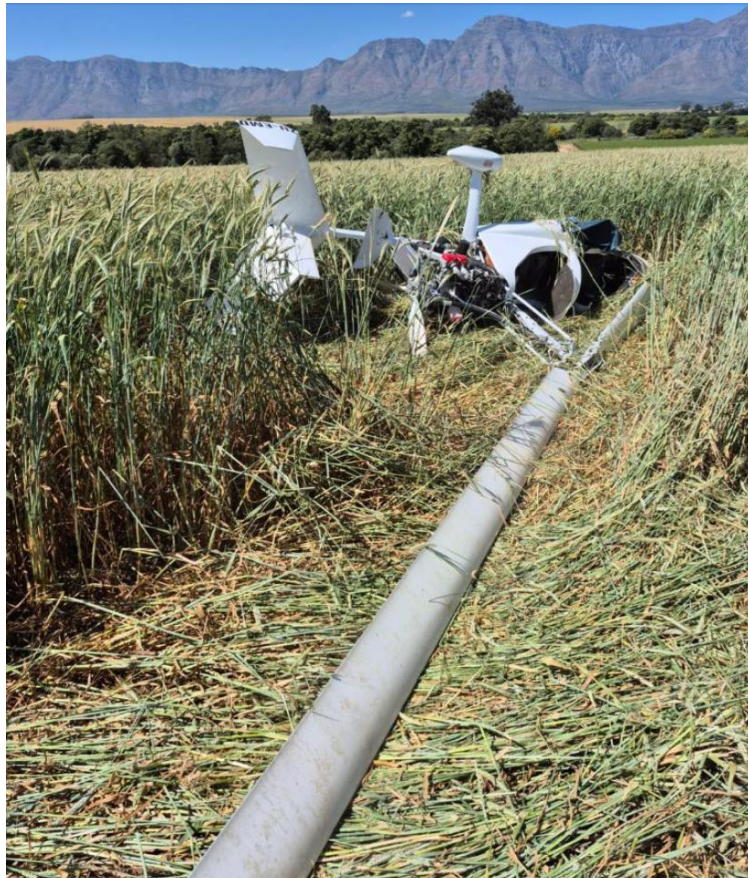
Figure 2: The Gyroplane at the accident site and the wheat crops cut by the rotor blades. (Source: Operator)
