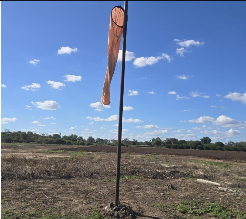
Figure 4: The windssock around the time of the accident; it indicated the absence of wind.
