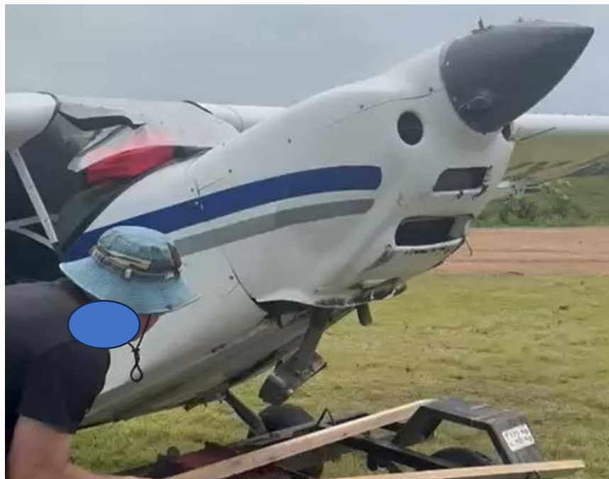
Figure 3: The damaged propeller blades and nose gear strut. (Source: Pilot)
