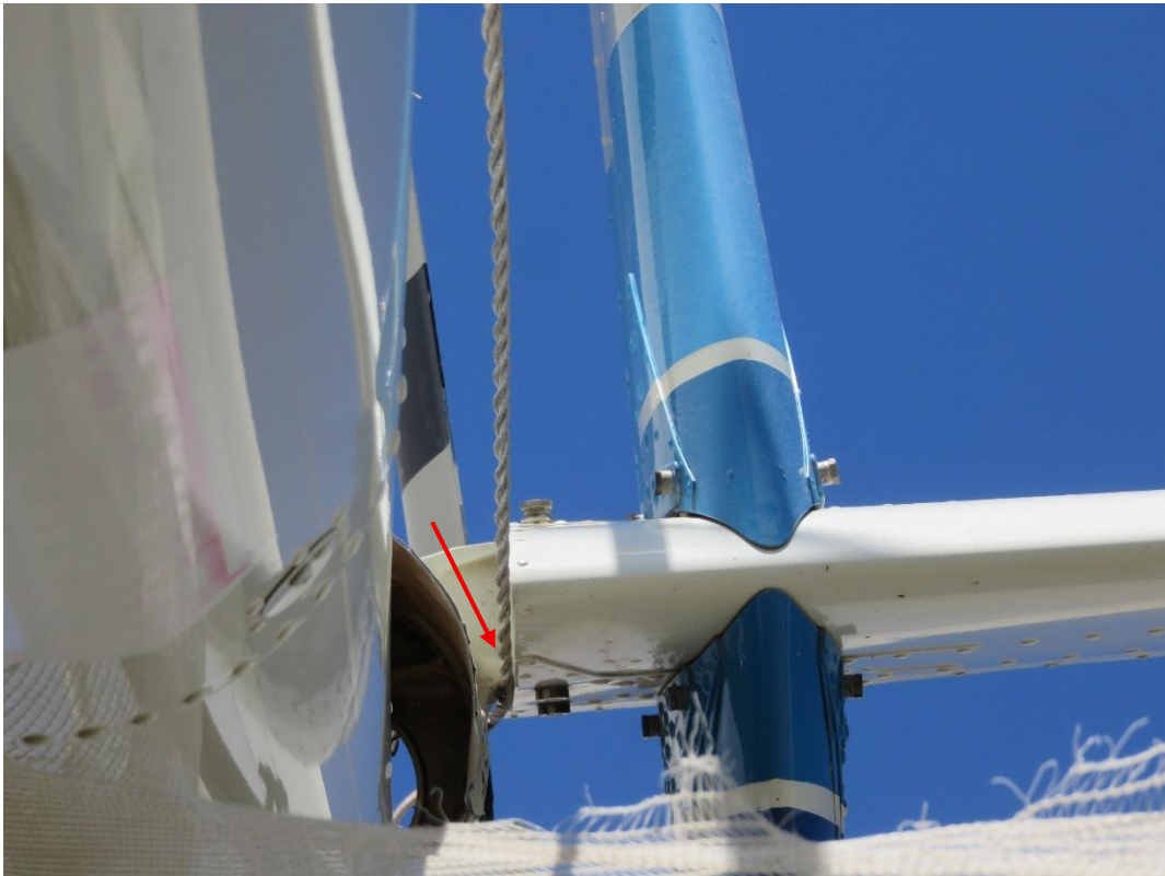
Figure 7: The cable was found hooked over the horizontal stabiliser.
