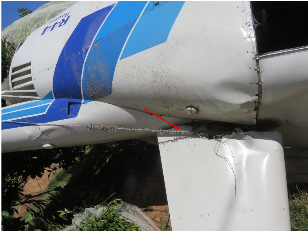
Figure 6: The cable entangled around the main rotor mast and control rods.
