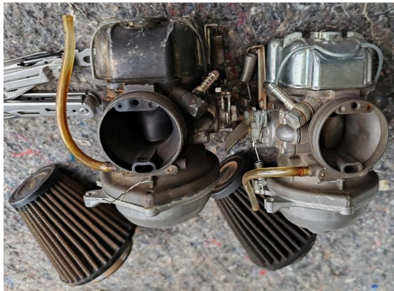
Figure 5: The left and right carburettors; the left carburettor shows carbon build-up.
