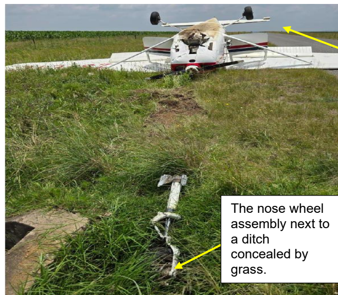
Figure 2: The final position of the aircraft in the background. The yellow arrow on the top right corner shows the direction of travel. In the foreground is the nose wheel that is stuck in a ditch. (Source: Operator)
