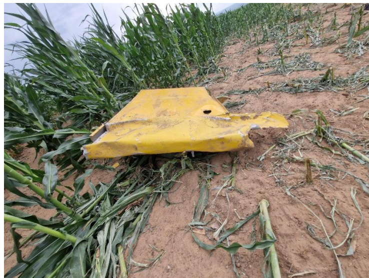
Figure 5: The left wing that impacted the ground and separated from the fuselage.
