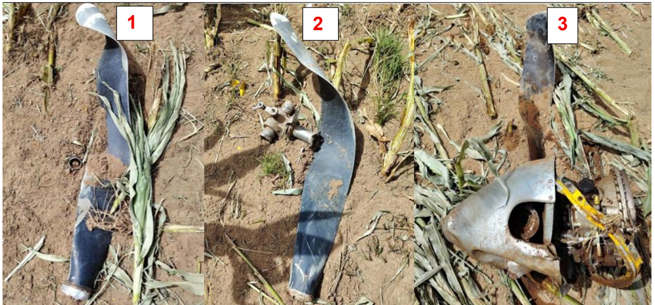
Figure 4: The three propeller blades indicate that the engine was producing power at the time of the accident.
