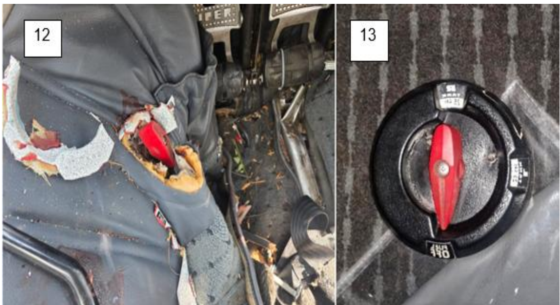
Figure 10: The fuel selector valve in OFF position (left).
