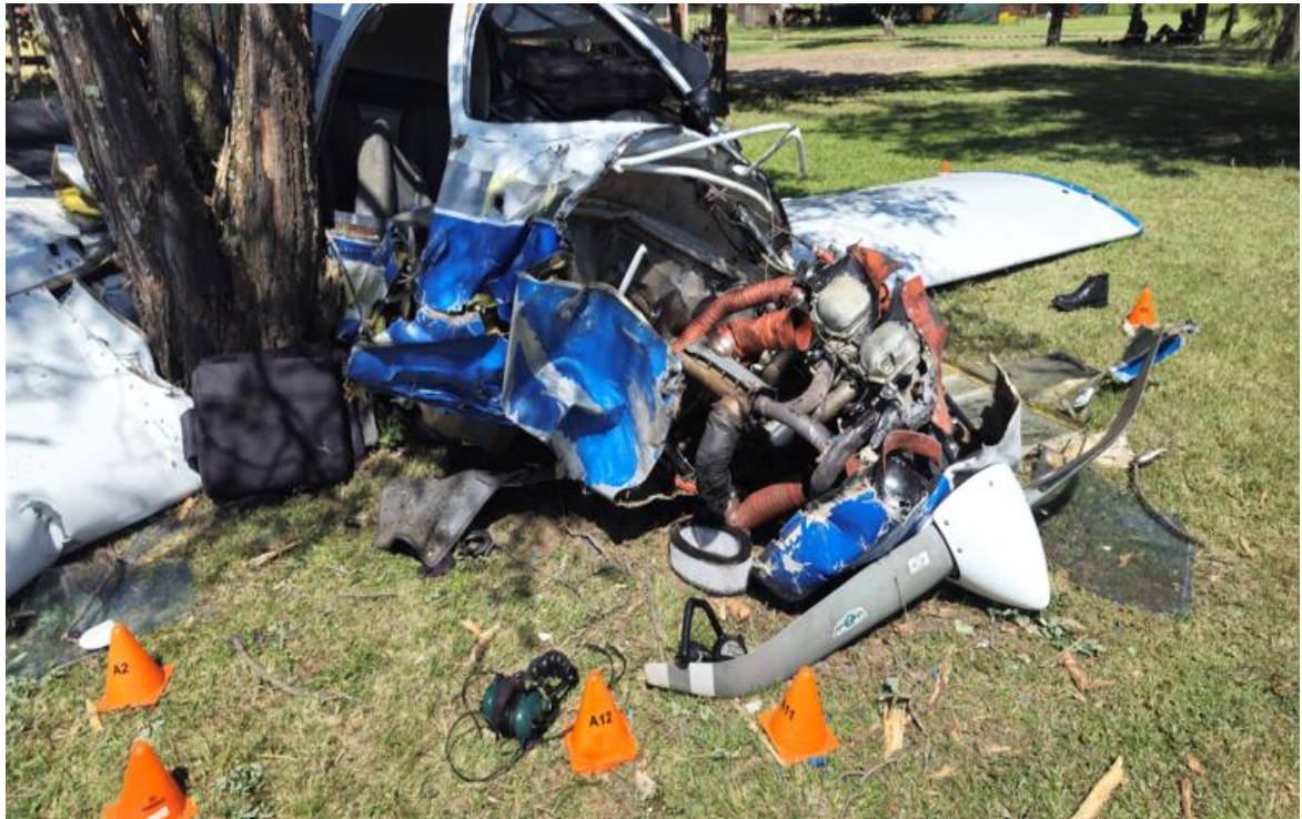
Figure 8: Damage to the engine compartment, engine mountings and the right wing.
