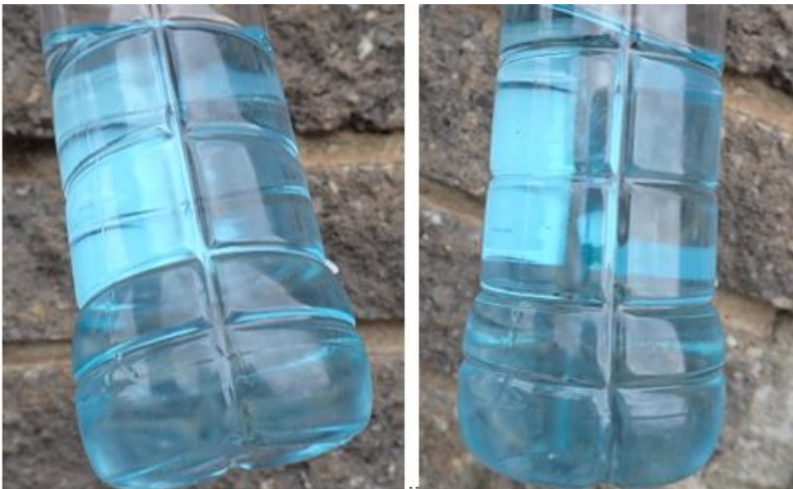
Figure 7: Fuel samples taken from the left and right header tanks.
