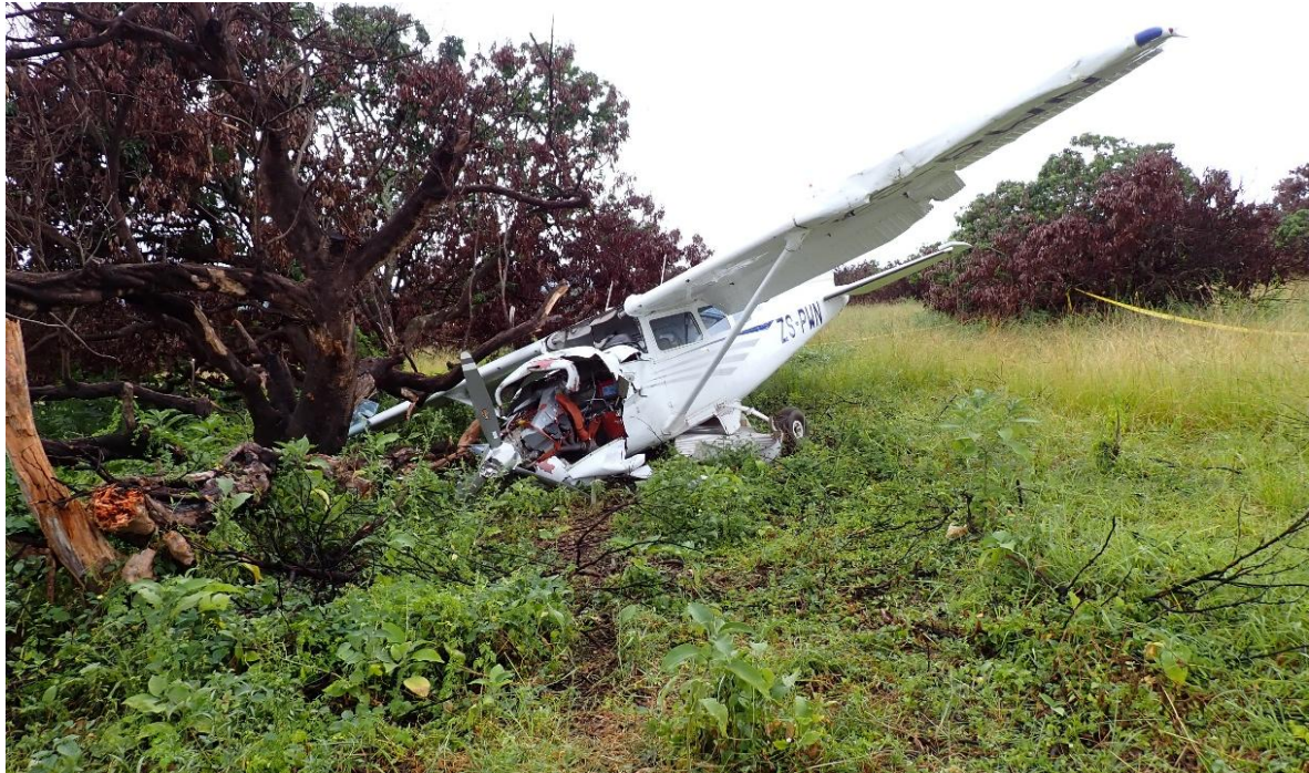
Figure 2: The aircraft after impacting a tree following a forced landing.
