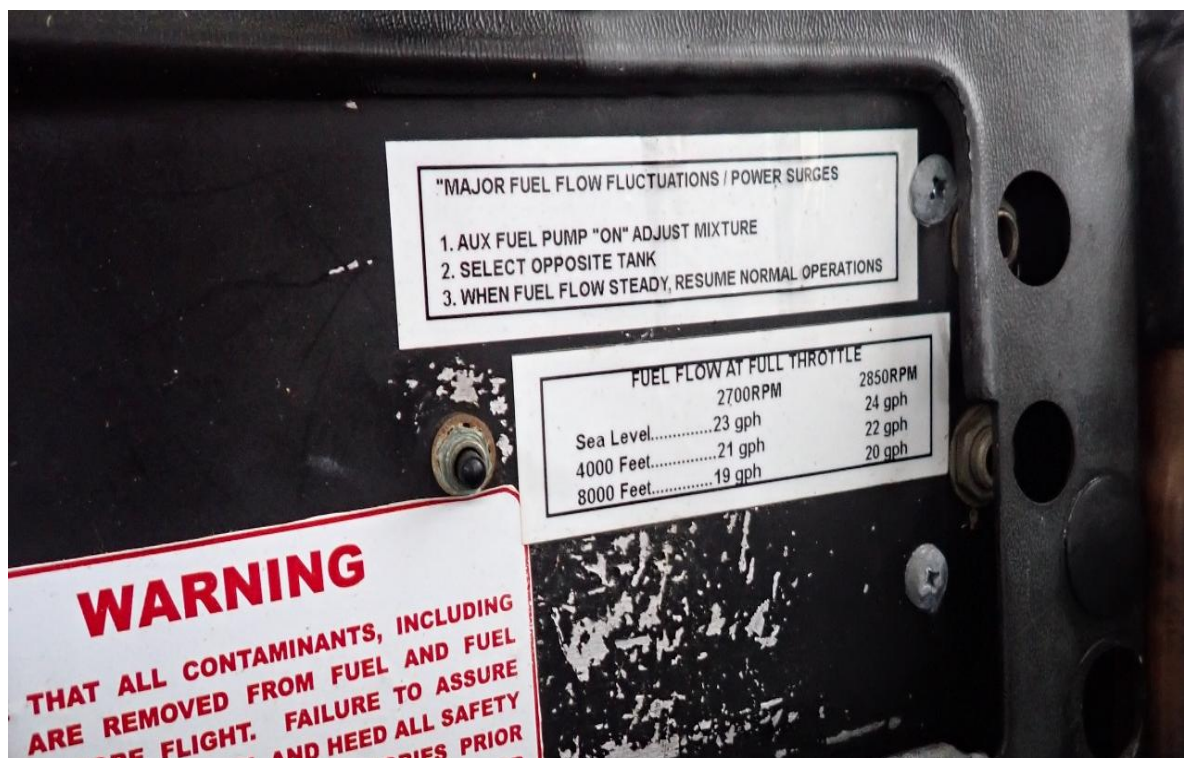
Figure 14: The fixed placard that was on the instrument panel of ZS-PWN as required by the Cessna SIL and the FAA AD 79-15-01.
