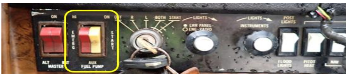
Figure 13: The auxiliary fuel pump switch in the cockpit of ZS-PWN.
