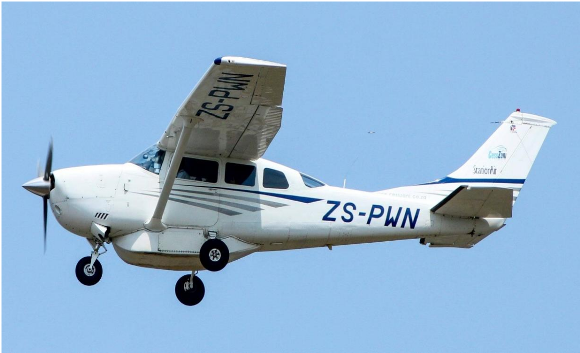
Figure 3: The ZS-PWN aircraft with the cargo pod installed. (Source: Operator)
