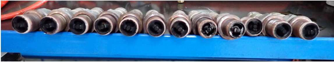
Figure 9: The heavily fouled 12 spark plugs.
