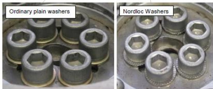
Figure 2 - Plain washers compared to Nordloc washers (flywheel with steel centre).
