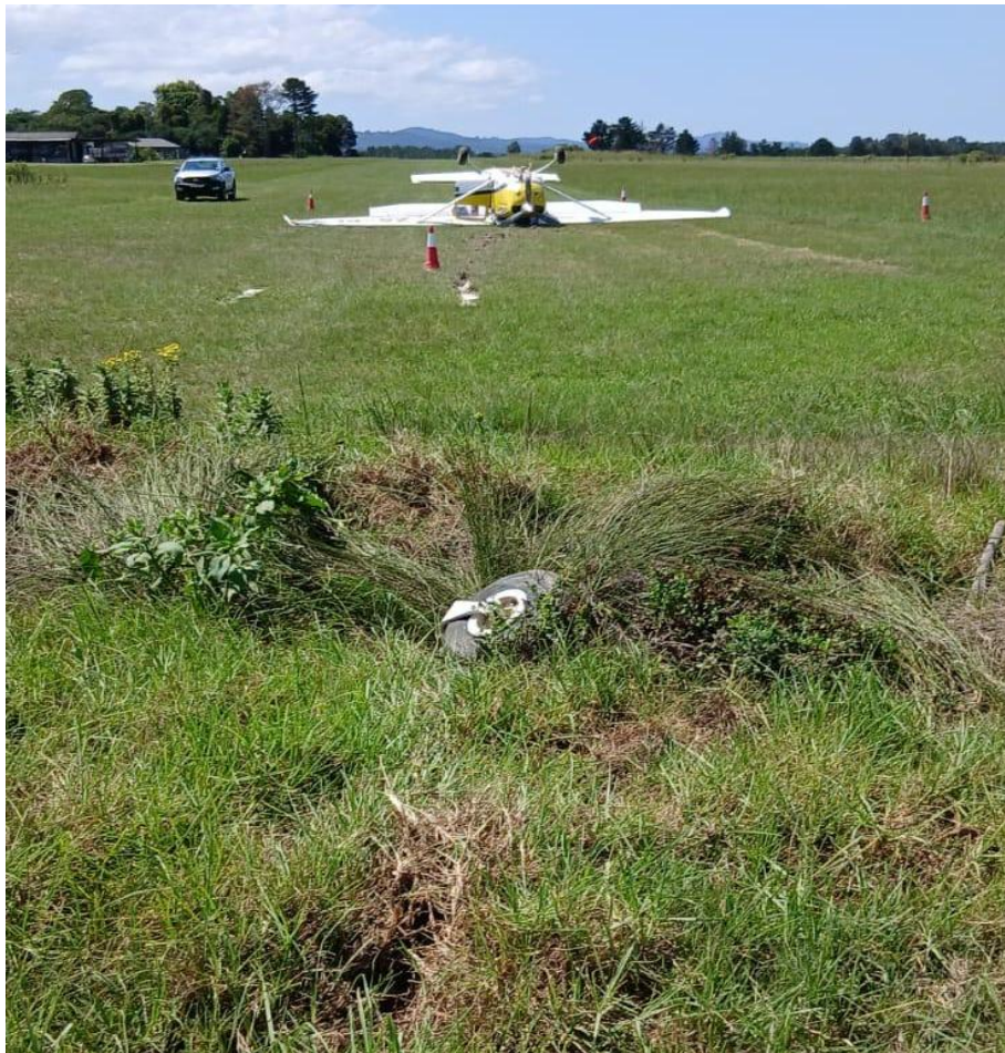
Figure 7: The area where the nose wheel assembly broke off. (Source: Incident Commander)
