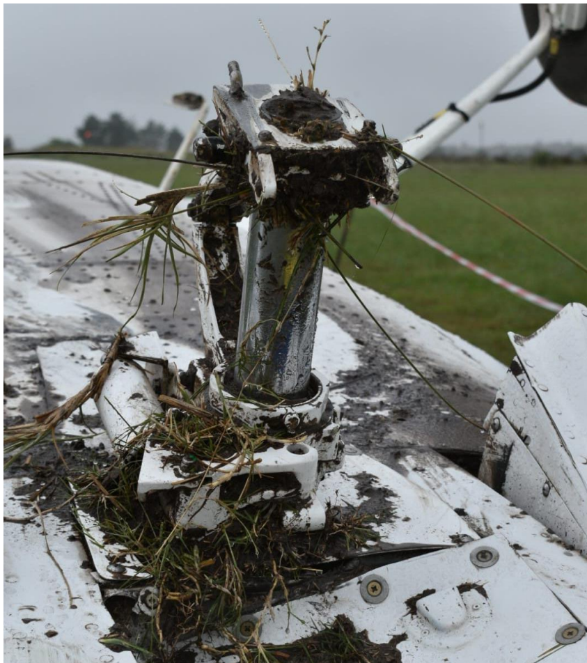
Figure 5: The nose gear oleo strut assembly that dug into the soft soil. (Source: Operator)
