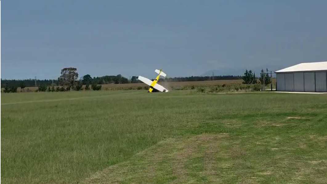
Figure 6: Snapshot from the video footage showing the dug-in left-wing tip as the aircraft nosed over. (Source: Incident Commander)
