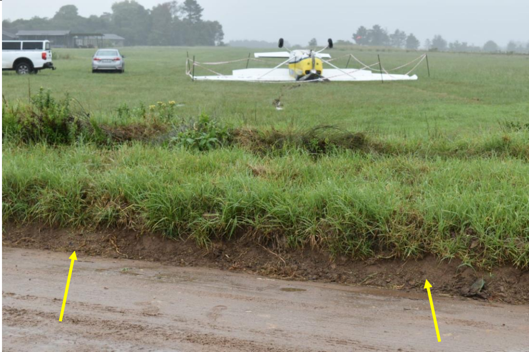
Figure 4: The embankment next to the road impacted by the main wheels. (Source: Operator)
