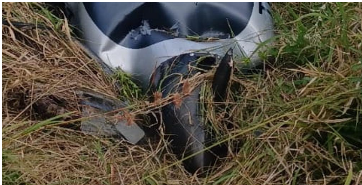
Figure 7: The fractured and separated propeller blade roots.
