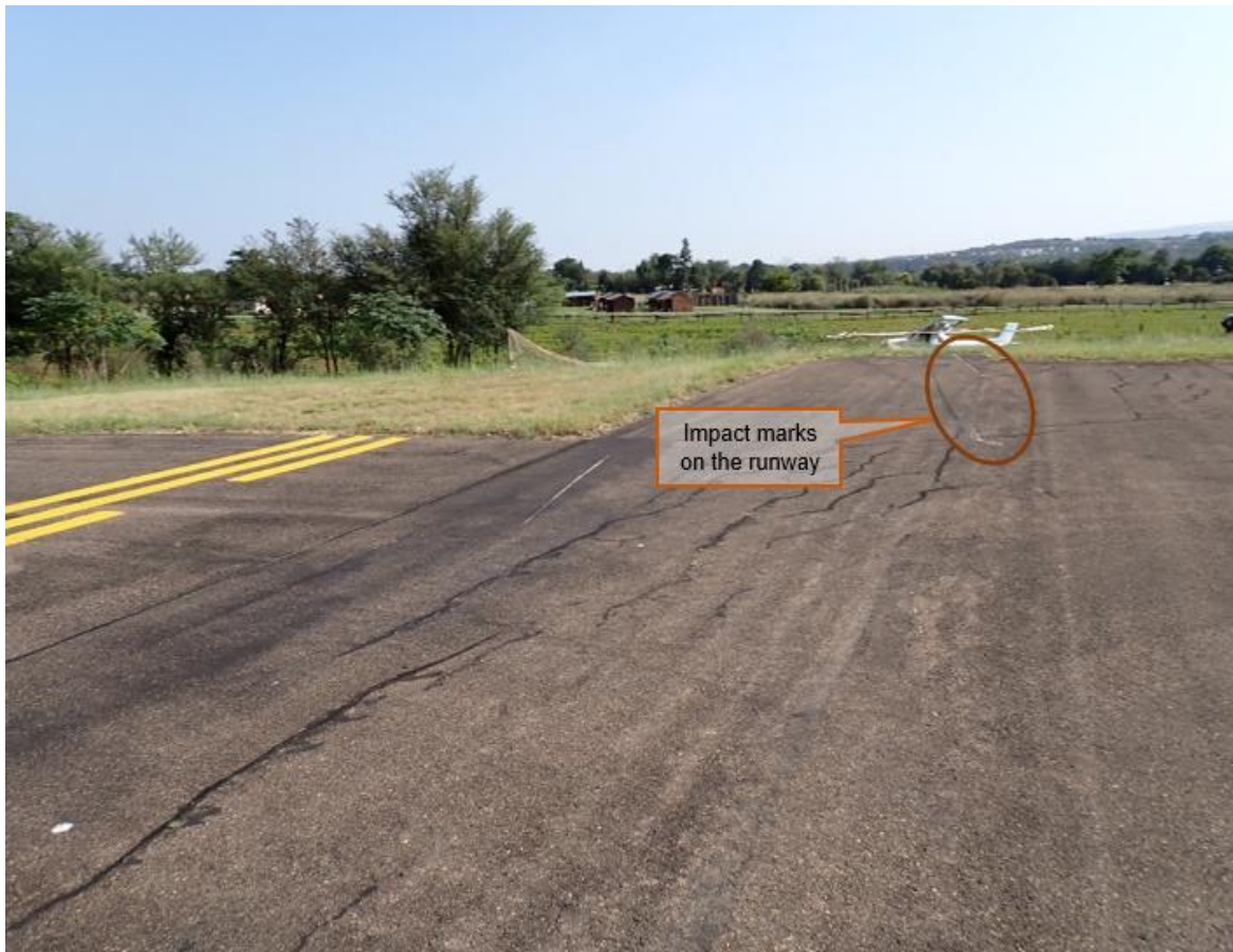
Figure 2: Impact marks on the runway with the aircraft in the background.
