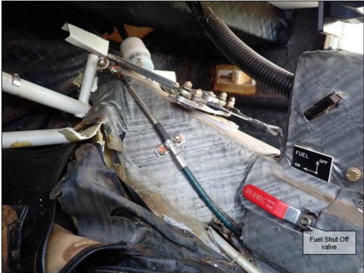
Figure 6: The fuel shut-off valve was found in open (ON) position.
