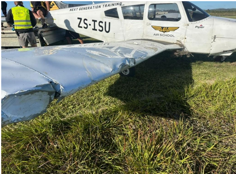
Figure 5: The damaged right wing. (Source: Operator)
