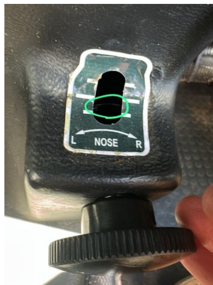
Figure 9: The trim control indicator as it was found set to the right. (Source: Operator)
