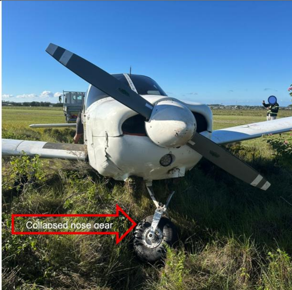
Figure 4: The collapsed nose gear. (Source: Operator)
