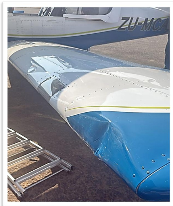
Figure 2: Damage to the left-wing leading edge.
