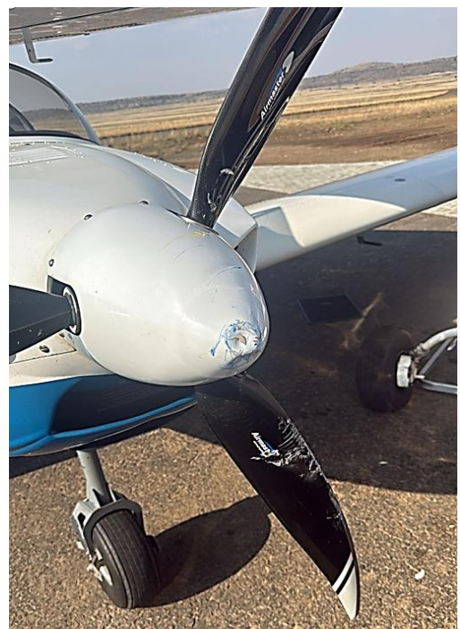
Figure 3: Damage to the propeller blades and spinner.
