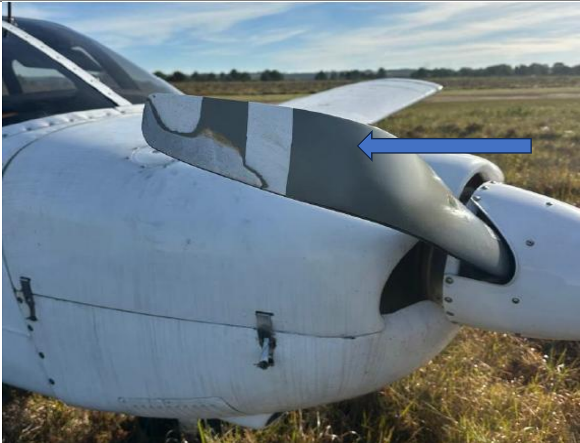
Figure 3: The blue arrow points to the damaged propeller blade. (Source: Operator)
