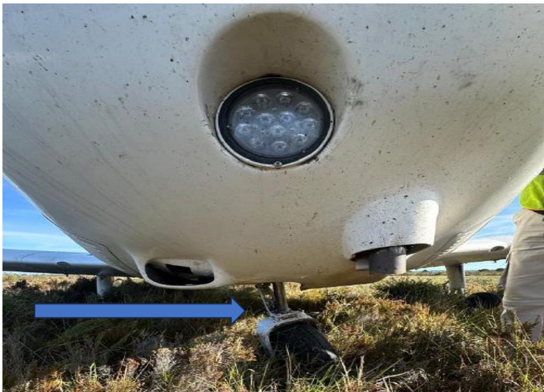
Figure 4: The arrow points to the damaged nose gear. (Source: Operator)
