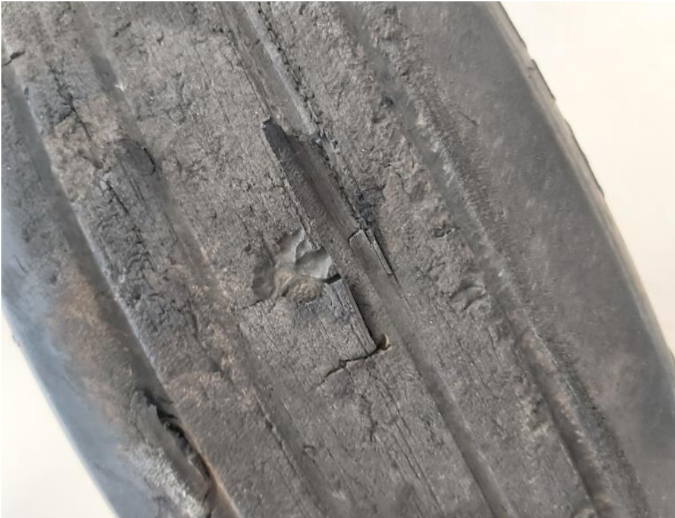
Figure 2: Wear damage on the left-side outboard tyre. (Source: AMO)
