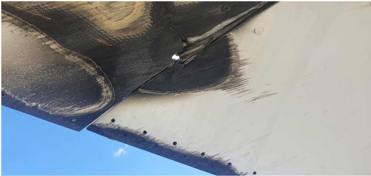
Figure 2: Underside damage on the right-wing tip.
