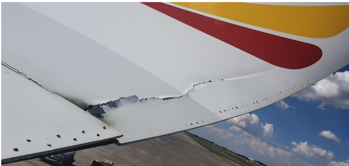
Figure 3: Upper side damage on the right-wing tip and winglet.
