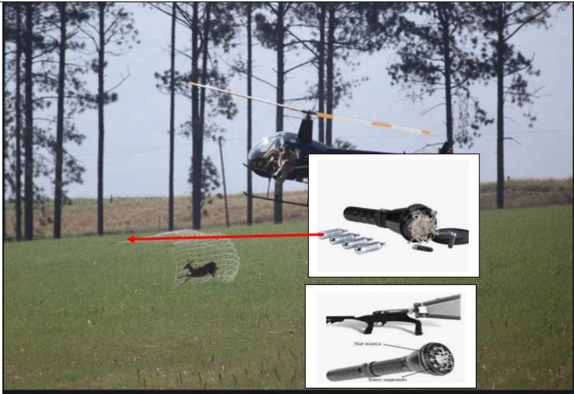
Figure 3: Demonstration of the net gun. The inset pictures show the net weights. (Source: https://www.helicopterwildlifeservices.com/wildlife-services/ and https://www.pecosales.com/product_pages/products.php?mi=79353&itemnum= )
