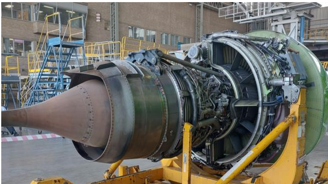
Figure 2: The damaged engine after it was removed from the aircraft.
