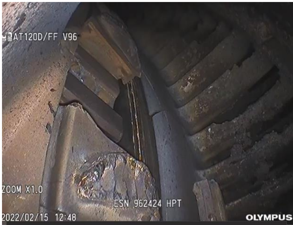
Figure 3: All blades sheared off. Two blades broke out of disk. (Source SAAT)
