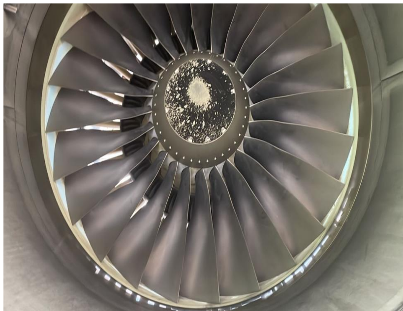
Figure 4: No damage to the compressor fan blades.
