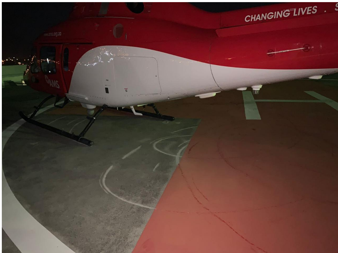
Figure 2: The scrape marks on the helistop made by the skids of the helicopter. (Source: Operator)
