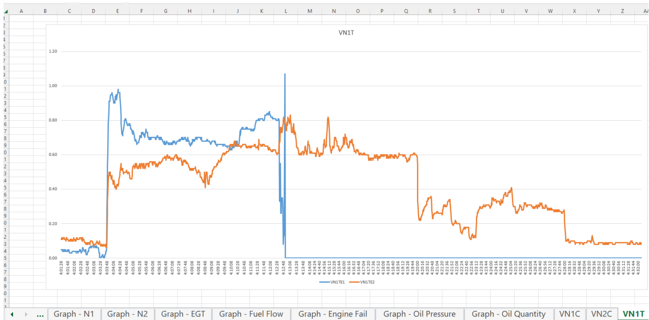
Graph 1: Blue line shows left engine VN1T and yellow line depicts right engine VN1T.
