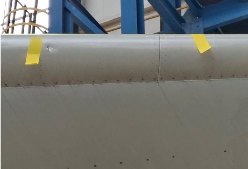
Figure 24: Damage to the leading edge of the left horizontal stabiliser.
