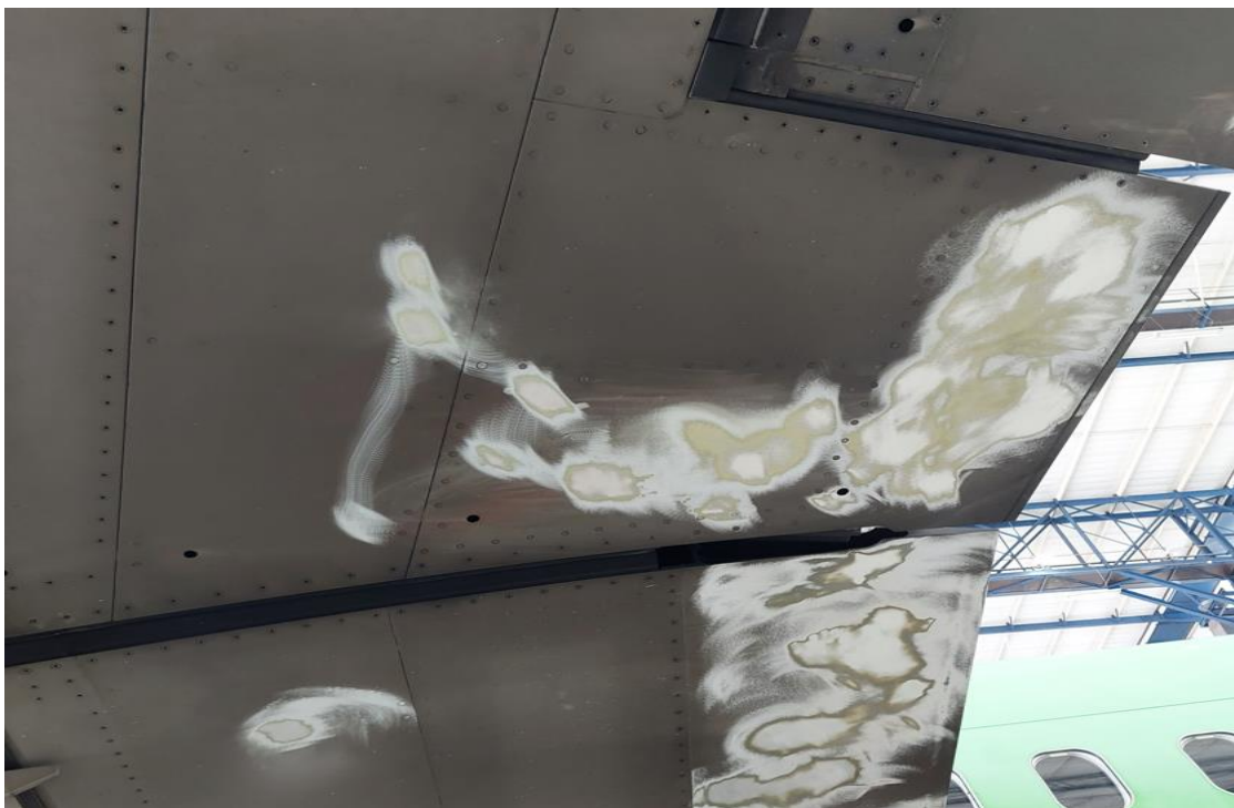
Figure 19: Inboard flaps during repairs.
