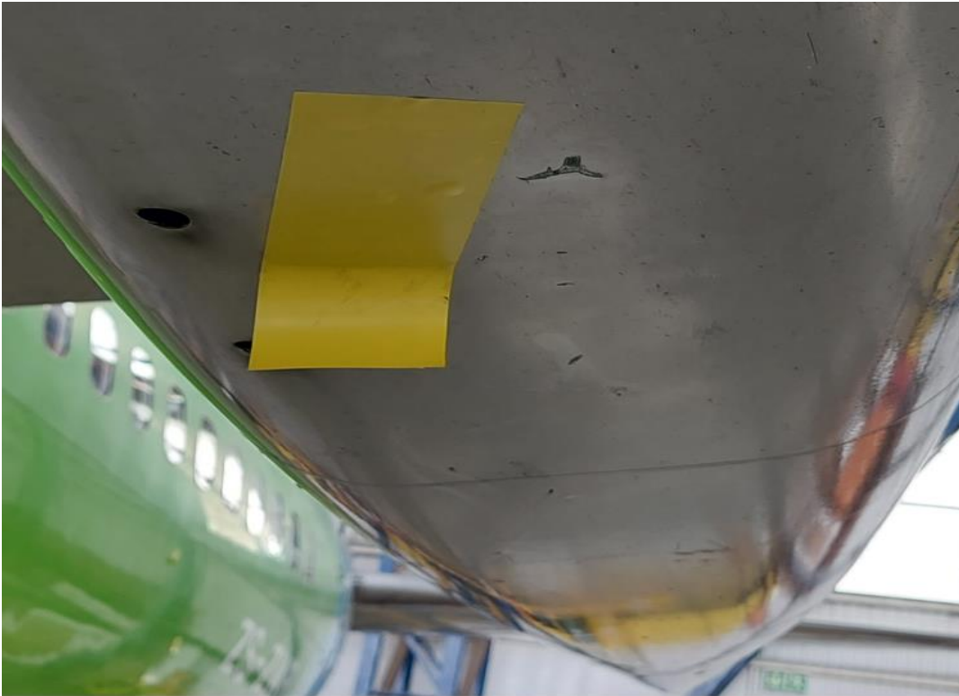
Figure 26: Damage to the underside of the fuselage aft section.
