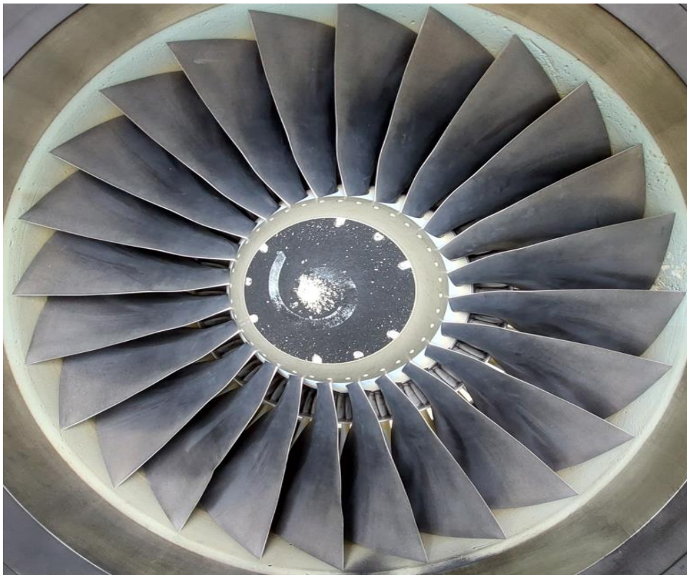
Figure 20: No damage to the fan blades.
