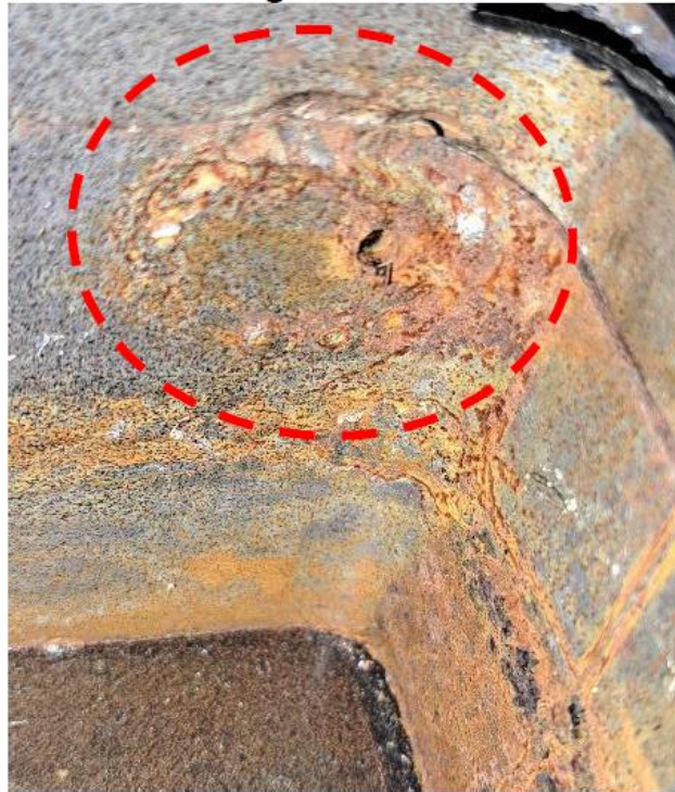
Figure 8: Inner tube area at fracture initiation point. (Source: University of Pretoria Report)
