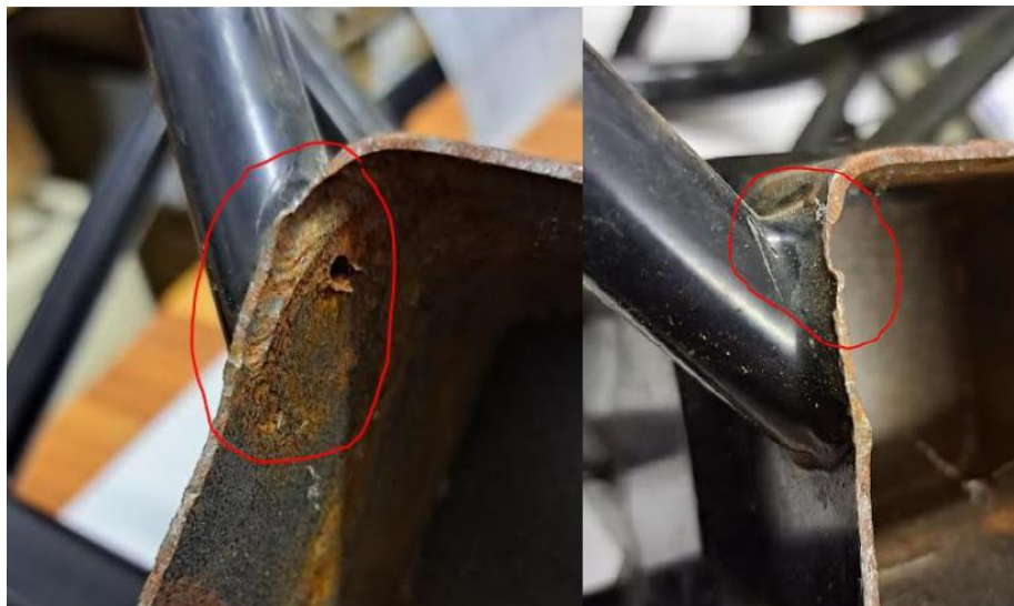
Figure 7: Engine mount fracture location. (Source: University of Pretoria Report)
