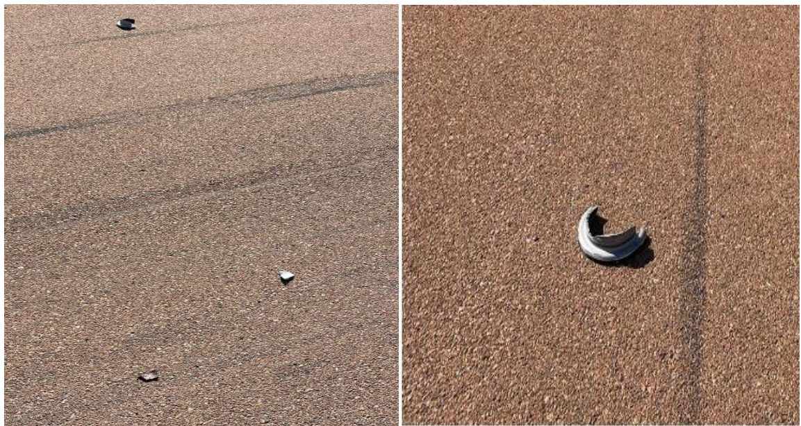
Figures 2 and 3: Left and right nose wheel hub debris. (Source: Operator)
