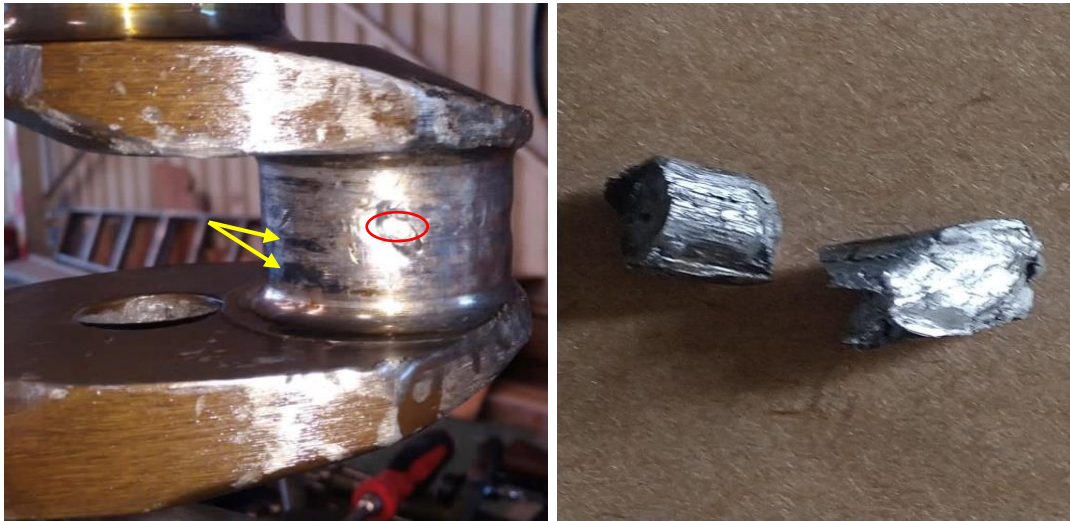
Figures 7 and 8: The crankshaft journal surface showing a blocked oil supply hole (red circle) and discolouration (left picture). The non-metal debris extracted from the hole (right picture). (Source: AMO)
