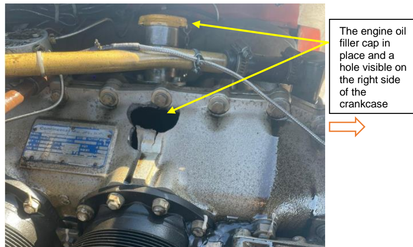
Figure 3: A hole on the right crankcase and the oil filler cap. (Source: AMO)
