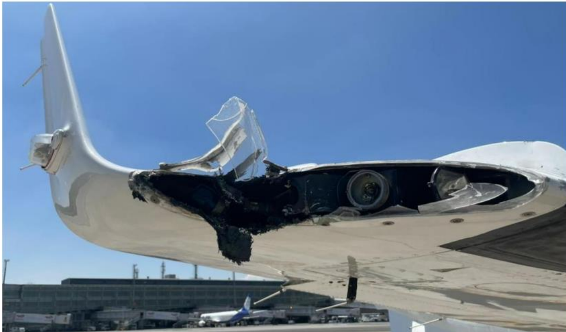
Figure 2: The damaged wingtip.
