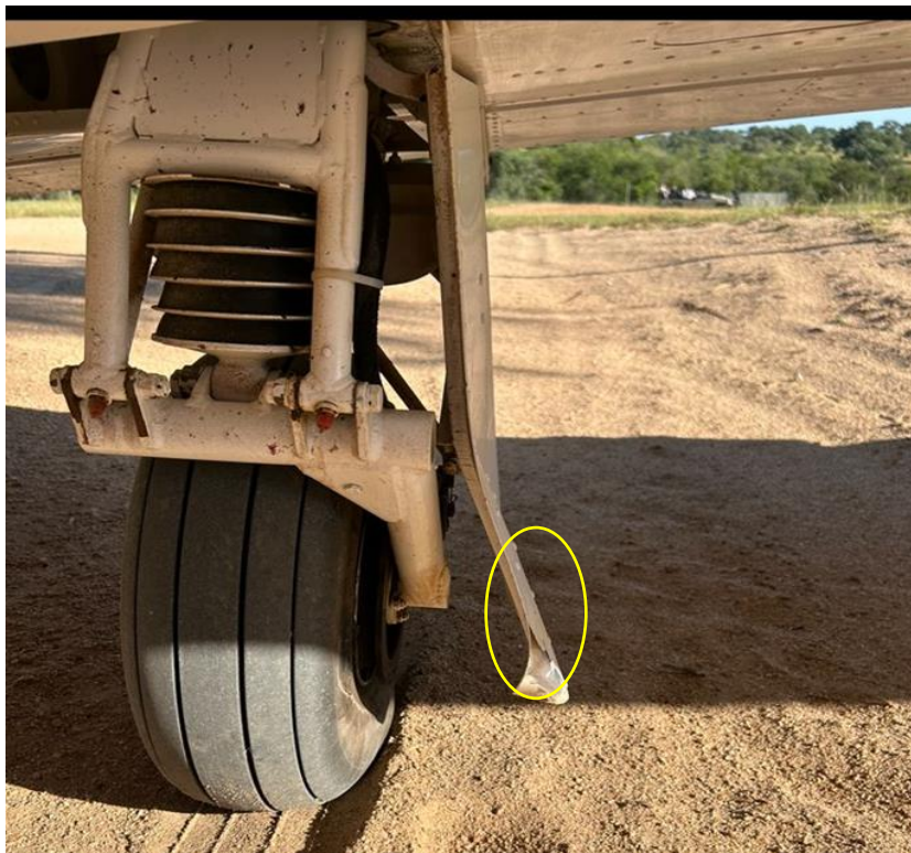
Figure 2: The damaged left main gear door. (Source: Pilot)
