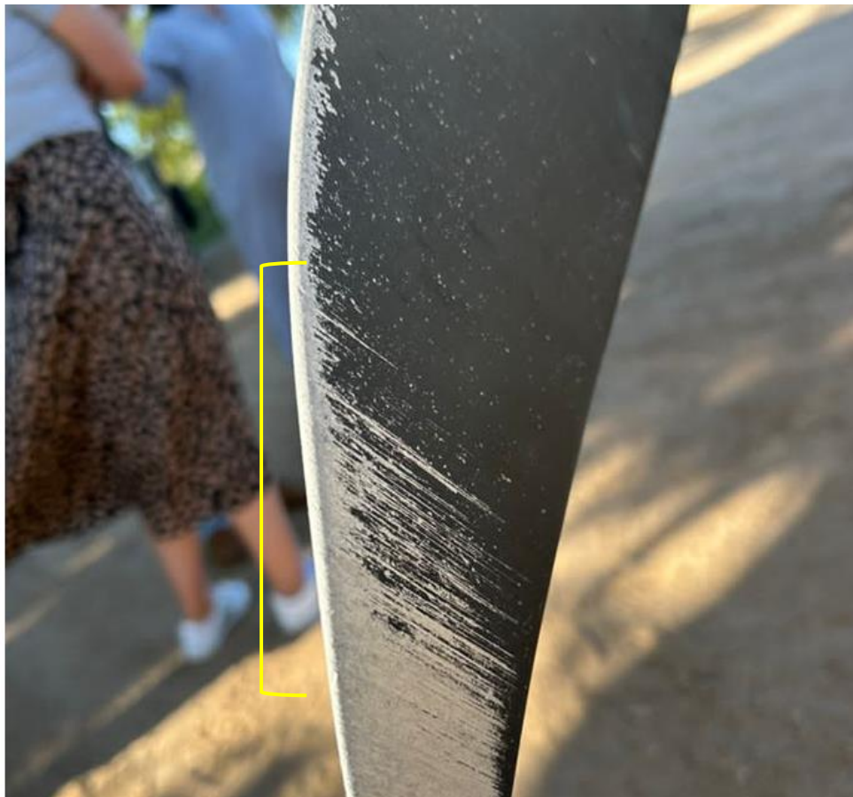
Figure 4: The bent propeller blade. (Source: Pilot)
